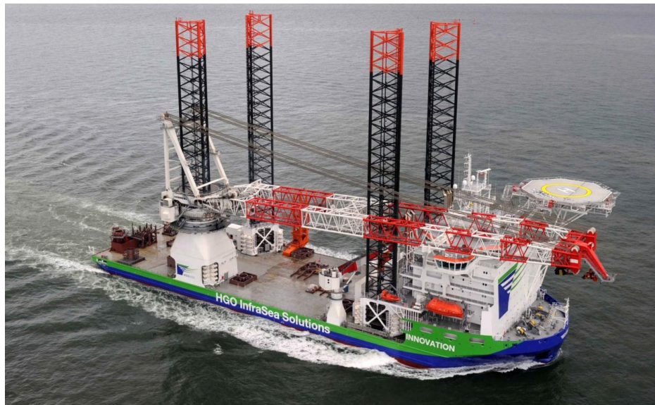
Figure 1.4: Jack-Up Vessel Innovation from HGO InfraSea Solutions
