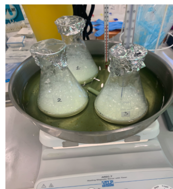
Figure 7: Heating set up with oil bath.
