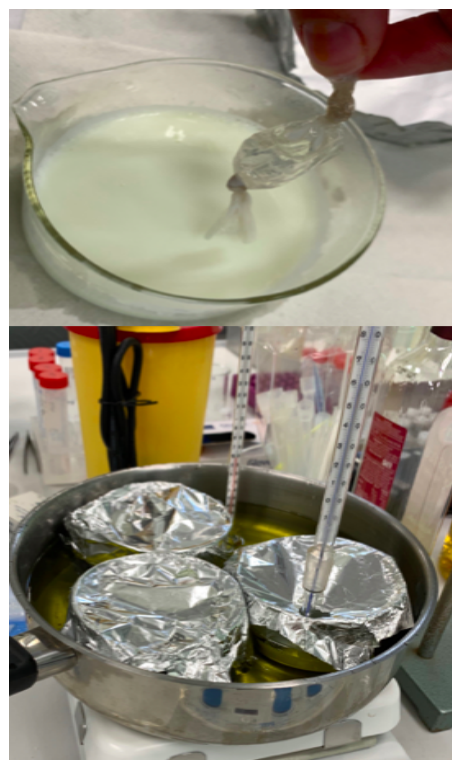
Figure 9: Figure A (top) shows how the membrane is prepared for heated dialysis and figure B (bottom) shows the dialysis set-up for heated dialysis.
