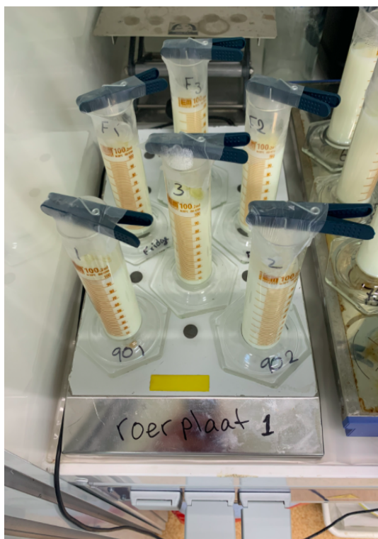
Figure 8: Dialysis set-up for room temperature dialysis
