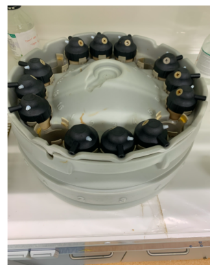
Figure 10: Microwave carousel with 12 microwave tubes evenly spread around the carousel. An even spread of the tubes is necessary for the microwave to run.
