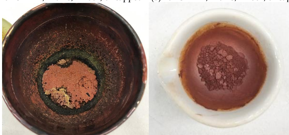
(c) 20\text{ }^{\circ}\text{C}\cdot\text{min}^{-1} , 220\text{ }^{\circ}\text{C} , 1 hour, capped (d) 20\text{ }^{\circ}\text{C}\cdot\text{min}^{-1} , 220\text{ }^{\circ}\text{C} , 1 hour, capped, grinded product
