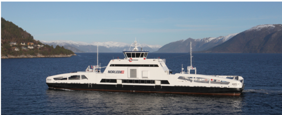
Figure 4.2: MF Ampere, full electric ferry [40]
