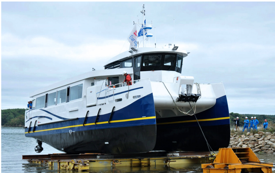
Figure 4.5: Ar Vag Tredan: supercapacitor powered ferry [20]
