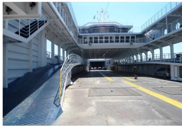
Figure 2.4: Ferry with side ramp [ 42 ]
