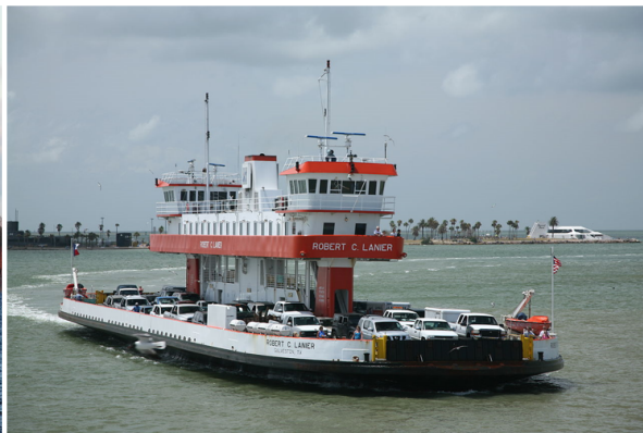
Figure 2.6: Ferry with central superstructure [ 10 ]
