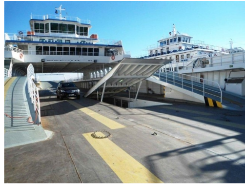
Figure 2.7: British Columbia ferry with double deck [27] Figure 2.8: Double bottom car deck [42]
