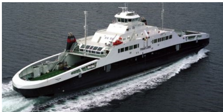
Figure 6.8: Ferry with a semi-open superstructure
