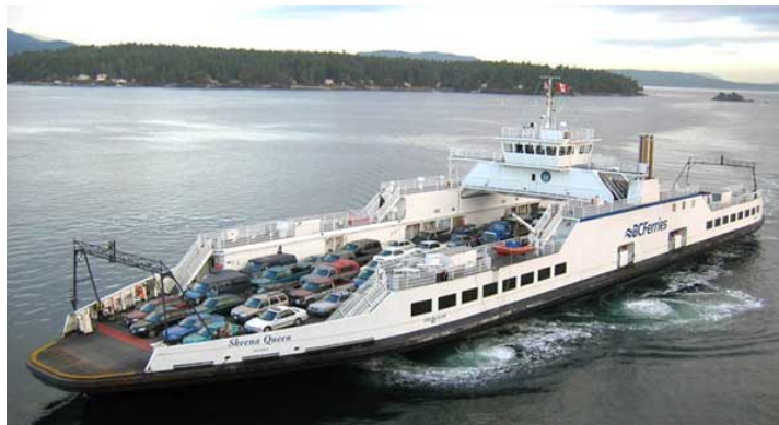
Figure 6.7: Ferry with an open superstructure
