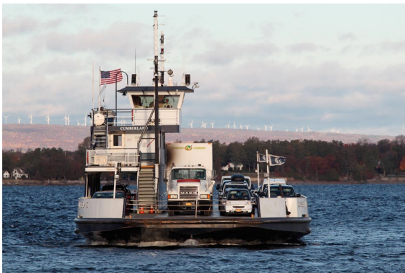
Figure 2.5: Ferry with open single sided superstructure [ 29 ]
