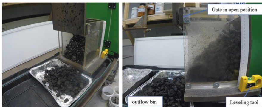
Fig. 4.18 Shear box test setup (Doorn, 2022). Reprinted with permission
