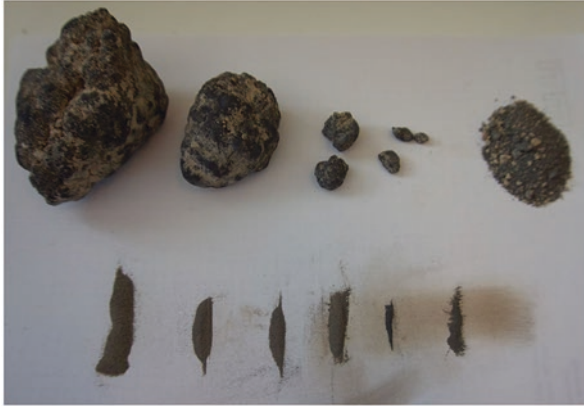
Fig. 4.15 Fragmented nodules and fines. (From: de Hoog et al., 2020. Copyright Elsevier 2020, reprinted with permission)
