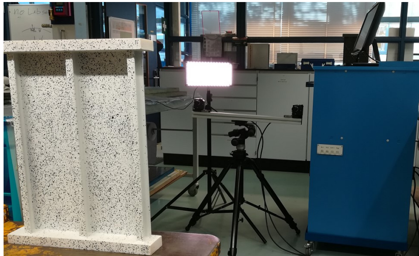
Figure 3: DIC measurement setup.
