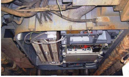
Fig. 24: Main converters container KHM 250 sub floor of tram T3 MOD 7304.
