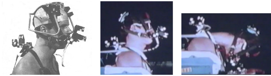
FIGURE 19.10 NBDL volunteer test configuration, instrumentation (left), posture at pulse onset (mid), and posture at maximum head rotation with 15G loading (right). NBDL , Naval Biodynamics Laboratory.
