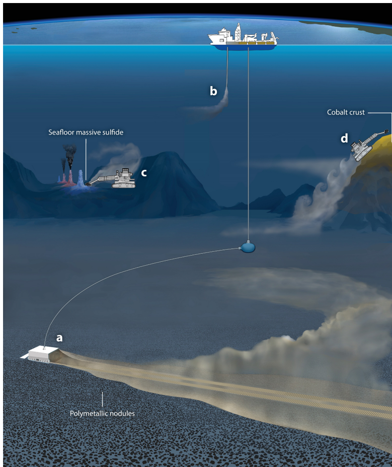
Figure 1.3: This illustration depicts three distinct types of proposed deep-sea mining activities, along with their associated sediment plumes (please note that the plumes and vehicles are not drawn to scale, and the mining operations are located in distant geographic areas). (a) A polymetallic nodule mining operation is shown using a single collector vehicle, and (b) a potential associated return water discharge. (c) A massive seafloor sulfide mining operation is depicted around a hydrothermal vent site. (d) Lastly, a cobalt crust mining operation is illustrated on the flank of a seamount. (Peacock and Ouillon, 2023).
