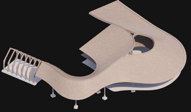
Structural Plywood Skin (In-situ applied 35mm plywood acts as a lateral restraint, creating a continuous structural support for timber ribs.)
