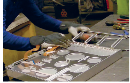
14. then a tool needs to be changed since the 4 th PCBA was also screwed to the LCD module
