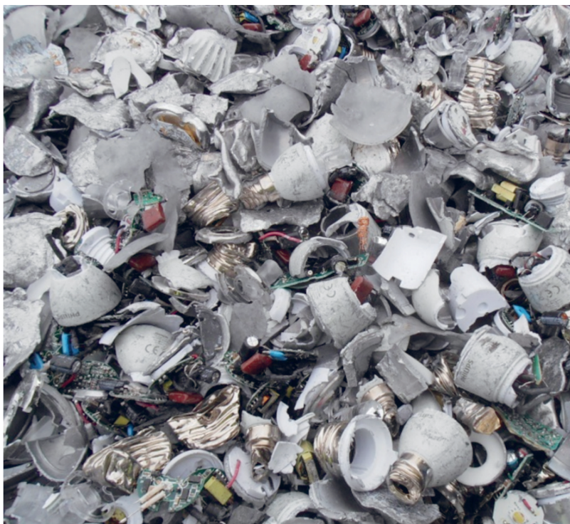
Figure 3.19- Close up of granulated bulbs. Image provided by Johan Felix, CIT Recycling Development AB.
