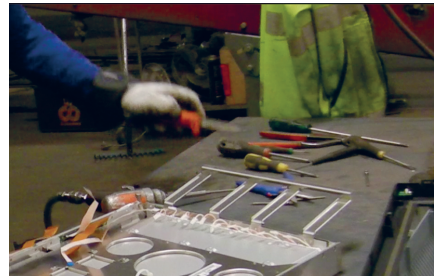
16. then a tool needs to be changed since complete removal of the 4 th PCBA was not possible even after removal of screws
