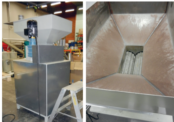
Figure 3.5- a: roller mill equipment, b: rotating rollers. Images provided by Johan Felix, CIT Recycling Development AB.
