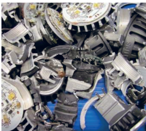
Figure 3.16- Spot lights fragments. Image provided by Johan Felix, CIT Recycling Development AB.
