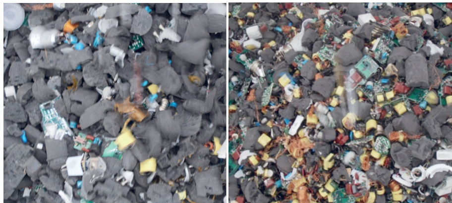
Figure 3.22-High-density fraction after wind sieve separation for LED bulbs in Run-1. Left: spots, right: bulbs. Images provided by Johan Felix, CIT Recycling Development AB.
