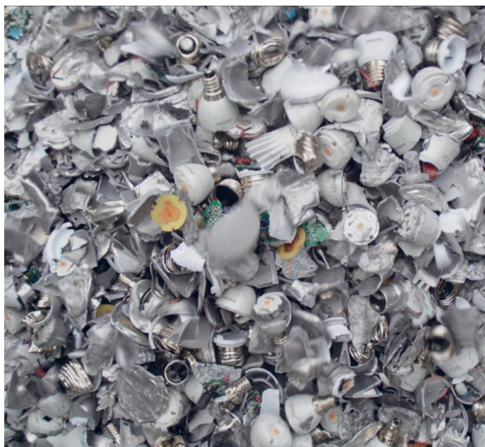
Figure 3.21-Aluminium fraction after eddy current separation for bulb LED lamps. Image provided by Johan Felix, CIT Recycling Development AB.
