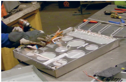
15. in total, eighteen screws are removed with power tool to partly release the 4 th PCBA
