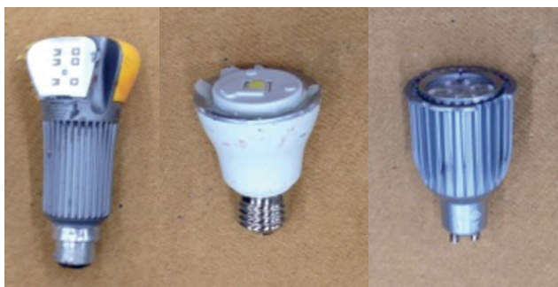
Figure 3.13-Example of LED lamps after a crush auger. Images provided by Johan Felix, CIT Recycling Development AB.
