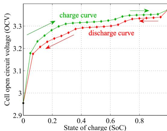
Figure 3.2: Typical Open Circuit Voltage hysteresis behaviour of a Lithium Iron Phosphate battery subject to a charge and discharge process at 20Ah [11]
