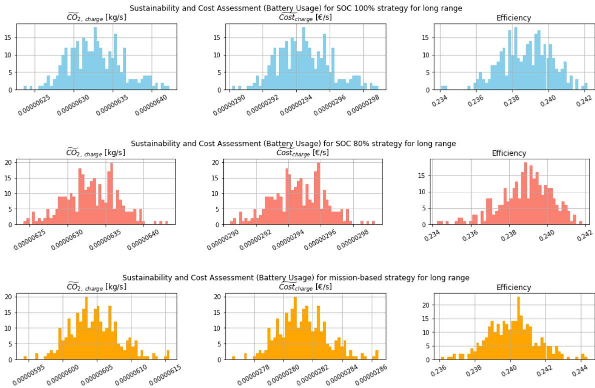
Figure 1.16: Distribution of Sustainability and Cost Assessment (Battery Usage) results of 300 batteries tested through Monte Carlo simulation for SOC 100%, SOC 80% and mission-based strategy for long range
