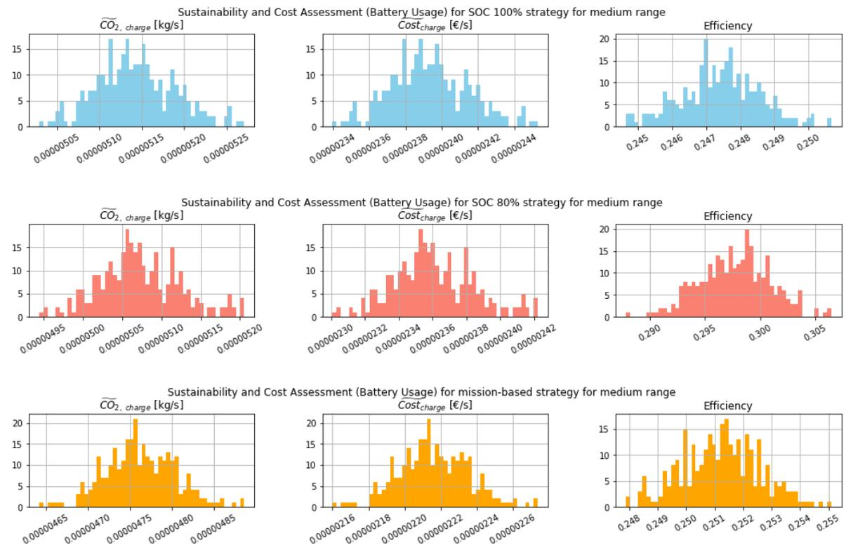
Figure 1.14: Distribution of Sustainability and Cost Assessment (Battery Usage) results of 300 batteries tested through Monte Carlo simulation for SOC 100%, SOC 80% and mission-based strategy for medium range
