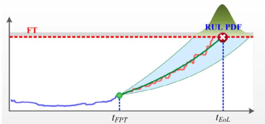
Figure 2.2: Determination of the Remaining Useful Life in Predictive Maintenance [74]
