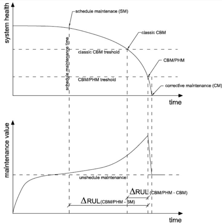
Figure 5.1: Analysis of value for different maintenance strategy levels [53]
