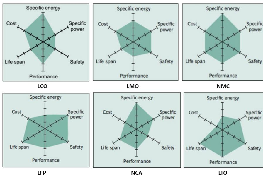
Figure 3.1: Hexagonal spider graphics of performance characteristics for Lithium-ion battery types LCO, LMO, NMC, LFP, NCA and LTO, showing specific energy, specific power, safety, performance, life span and cost [23]
