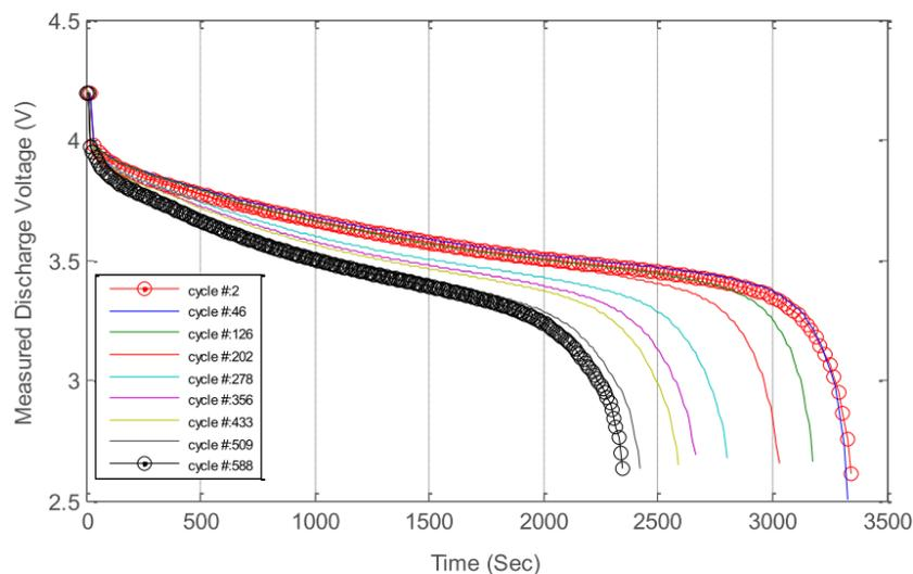
Figure 3.4: Discharge cycles at different battery life stages for constant load profiles from one single Lithium battery [112]
