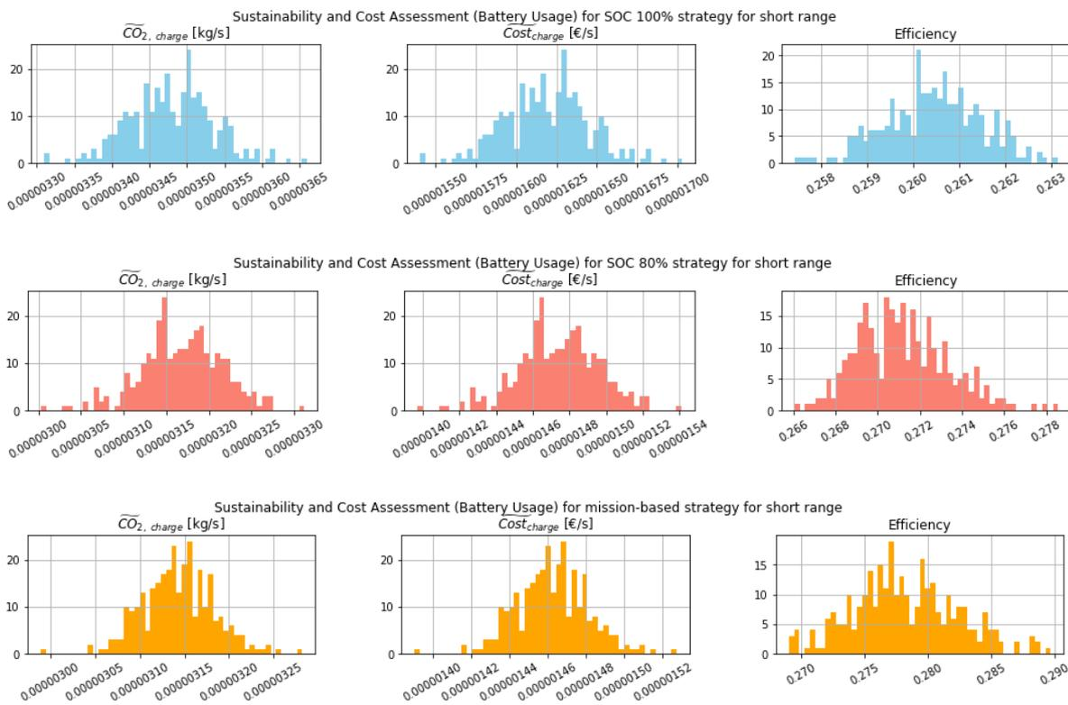
Figure 1.12: Distribution of Sustainability and Cost Assessment (Battery Usage) results of 300 batteries tested through Monte Carlo simulation for SOC 100%, SOC 80% and mission-based strategy for short range
