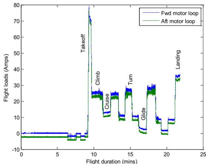
Figure 3.3: Typical eUAV flight load during flight [108]
