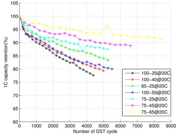
Figure 3.5: Lithium-ion battery capacity retention behaviour related to different Depth-of-Discharge ranges during battery Dynamic Stress Testing (DST) [132]
