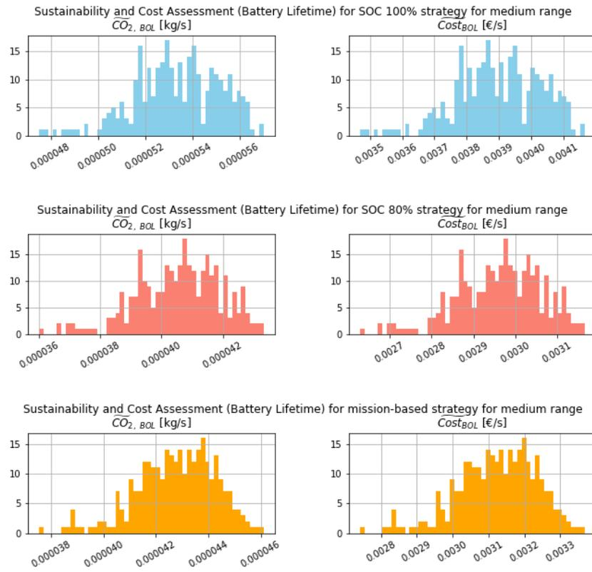
Figure 1.13: Distribution of Sustainability and Cost Assessment (Battery Lifetime) results of 300 batteries tested through Monte Carlo simulation for SOC 100%, SOC 80% and mission-based strategy for medium range
