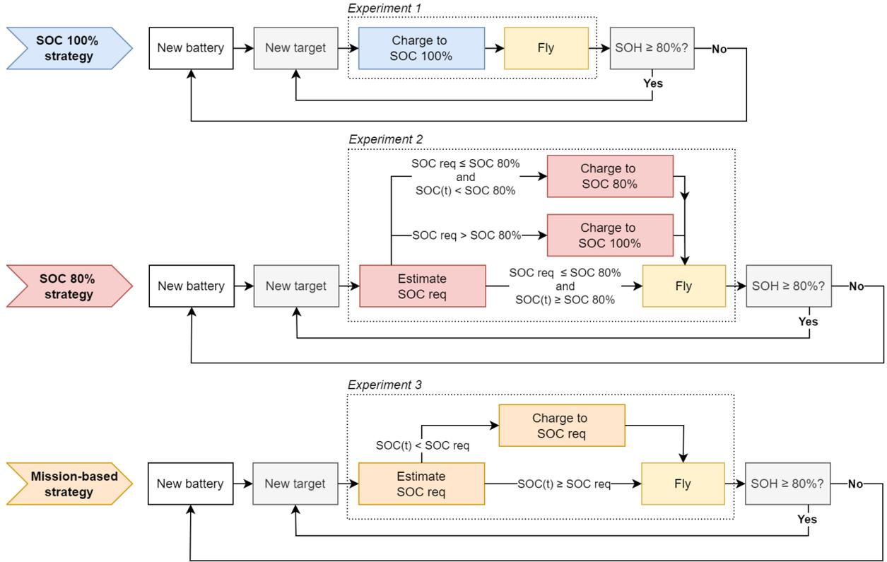
Figure 1: Schematic overview of SOC 100%, SOC 80% and mission-based strategy battery models
