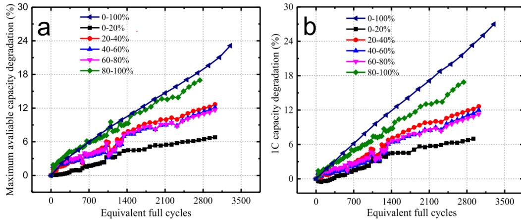
Figure 3.6: Lithium-ion battery capacity loss due to different Depth-of-Discharge ranges, showing (a) maximum available capacity degradation, (b) nominal capacity degradation [47]
