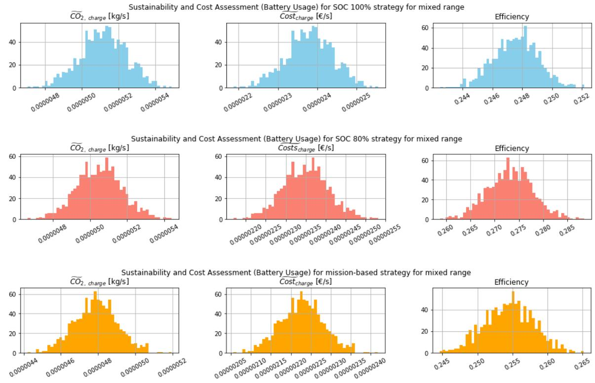
Figure 1.10: Distribution of Sustainability and Cost Assessment (Battery Usage) results of 1000 batteries tested through Monte Carlo simulation for SOC 100%, SOC 80% and mission-based strategy for mixed range
