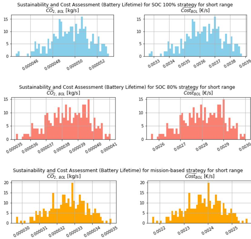
Figure 1.11: Distribution of Sustainability and Cost Assessment (Battery Lifetime) results of 300 batteries tested through Monte Carlo simulation for SOC 100%, SOC 80% and mission-based strategy for short range
