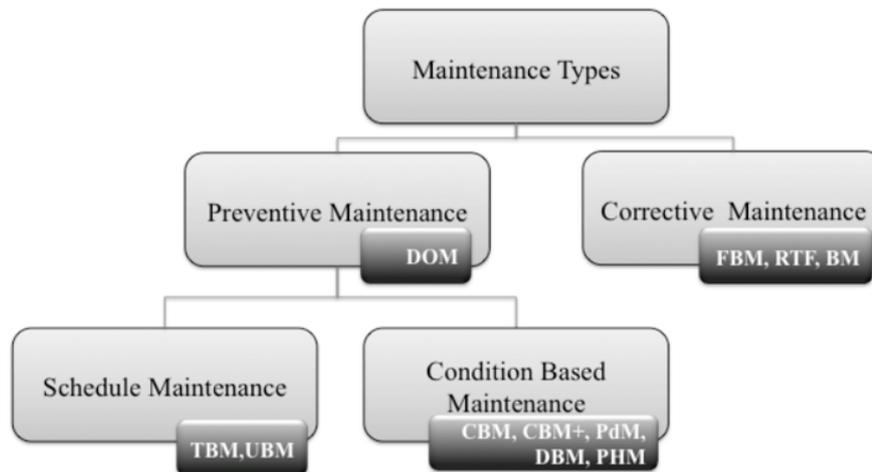
Figure 2.1: Breakdown Tree of Maintenance Types [53]
