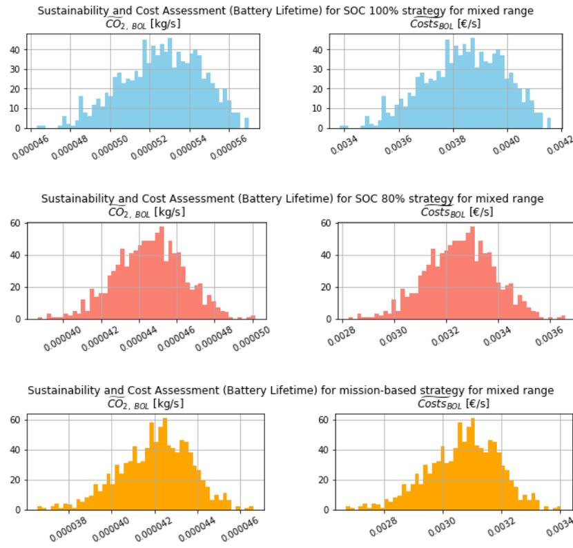
Figure 1.9: Distribution of Sustainability and Cost Assessment (Battery Lifetime) results of 1000 batteries tested through Monte Carlo simulation for SOC 100%, SOC 80% and mission-based strategy for mixed range
