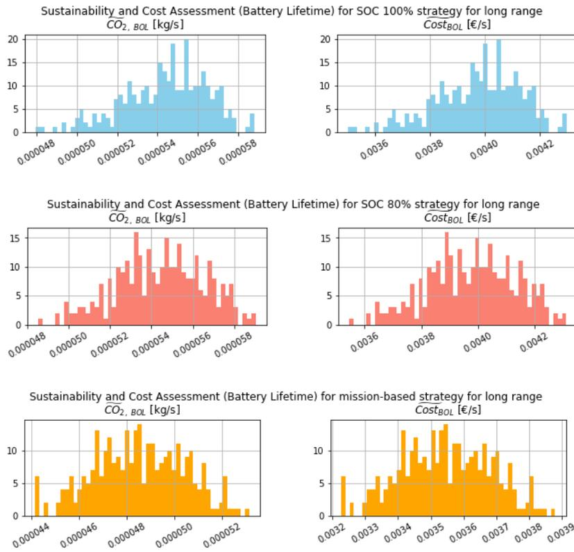
Figure 1.15: Distribution of Sustainability and Cost Assessment (Battery Lifetime) results of 300 batteries tested through Monte Carlo simulation for SOC 100%, SOC 80% and mission-based strategy for long range
