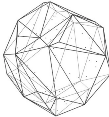
Figure 2.8.: Example of convex hull of 3D points (Lorie Toma's lecture slides [63]).
