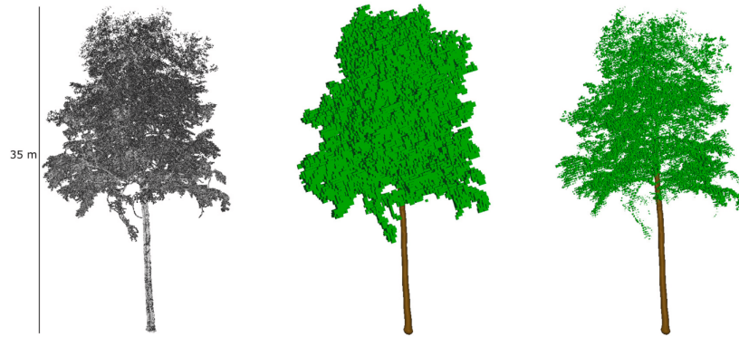
Figure 2.7.: Individual tree point cloud and two of its different representation (Weiser et al., 2021)
