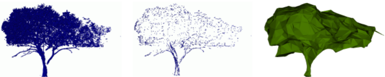
Figure 2.10.: Example of implementation of Zhu et al. (2008). From left to right: 1) original point cloud, 2) outer boundary points, 3) resulting boundary mesh model.
