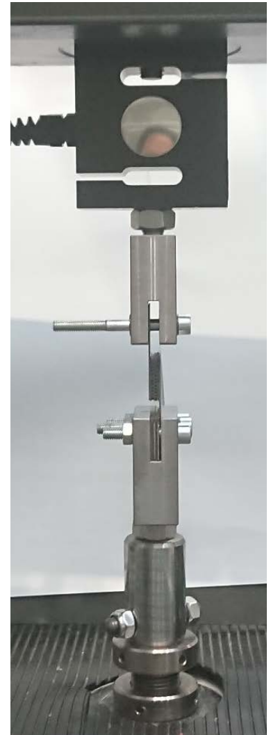
Figure 3: Single lap shear test setup used to measure the shear stiffness of the printed adhesive structures.
