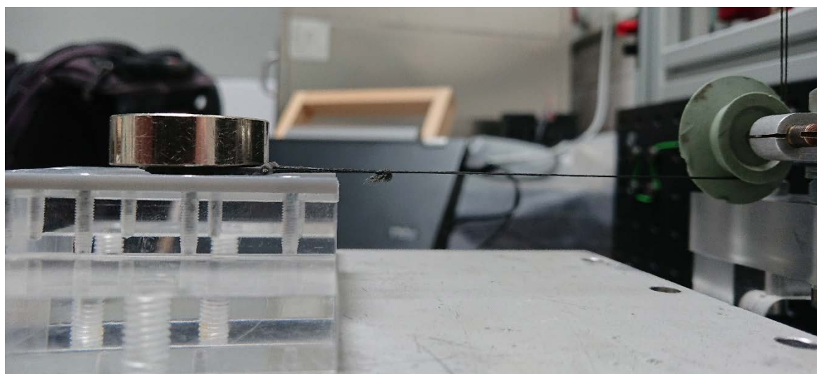
Figure 4 Upper right: the test setup used to test the adhesives on PVA substrates; the sample is aligned with the use of a small weight. Upper left: the test setup equipped with the glass slide and a piece of cloth clamped to the glass with the use of paper-clips; the alignment weight is removed from the sample and the normal preload is applied. Bottom: friction test on PVA.
