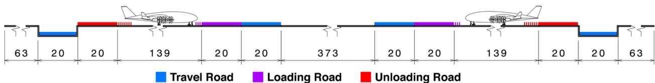
Figure 8.3.: Side view showing travel roads, loading roads (near nose) and unloading roads (near tail)
