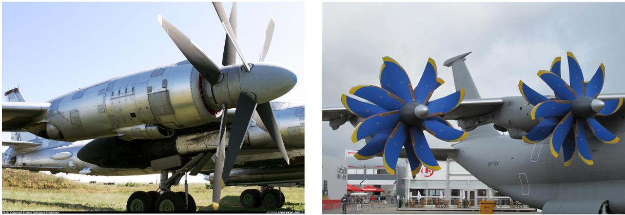
Figure 6.18.: NK-12 [49] and D-27 [50] Counter-Rotating Propeller Engines.
