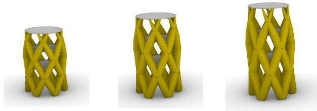
*Figure 125. Diagrid tree tower with storey height as the parametric variable*
