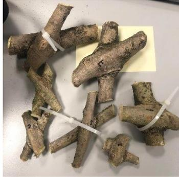
Figure 48. Crosswise connection specimens
