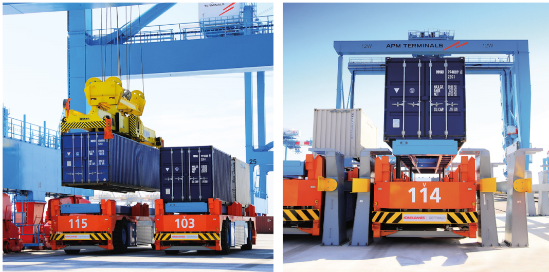
Figure 1.2: Lift-AGVs at Quay Crane transfer points (left) and at stack transfer points (right) [1].
