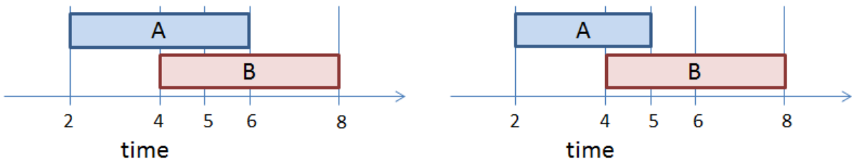
Figure 4.5: Schematic example of conflicting desired claim occupations of a certain area by A and B (left), and the same situation with a shorter occupation time of vehicle A (right). The shorter occupation of A leads to a higher relative priority value as the potential hindrance for B is decreased.
