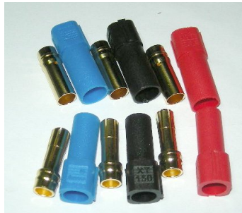
Figure 28.: The XT150 connector to detach the coil from hardware.
