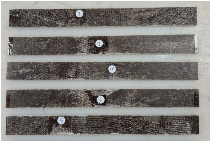
Fig. 7.2 Specimen 1-5 prepared for tensile testing (cross-stitched flax fibre cloth) (own image)
