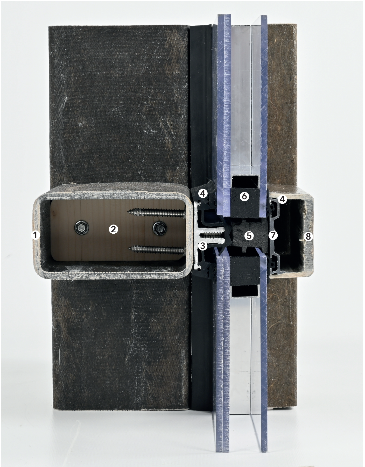
Fig. 8.29 Cross-section of façade model showing: (1) flax fibre-epoxy mullion and transom profiles, (2) timber connector profile, (3) aluminium base profile, (4) rubber sealing system, (5) insulation block, (6) glazing spacer, (7) aluminium pressure profile, and (8) hemp fibre-epoxy exterior cap (own image)
