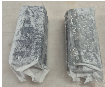
Fig. 6.14 Specimen 4 and 5 before demoulding (own image)
