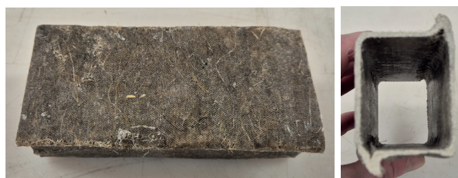
Fig. 6.16 Result specimen 4 using vacuum bagging, a peel-ply and a breather cloth (own image)
