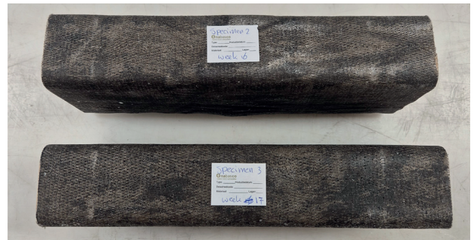
Fig. 8.19 Specimens 11 and 12 prepared for the three-point bending test (own image)
