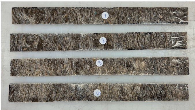
Fig. 7.3 Specimens 6-9 prepared for tensile testing (non-woven hemp fibre mat) (own image)
