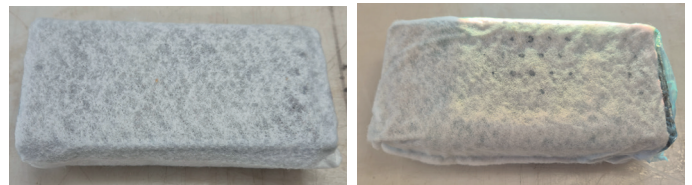
Fig. 6.22 Specimen 5 (left) and specimen 6 (right) out of vacuum bag with breather cloth (own image)
