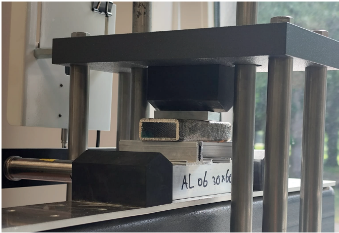
Fig. 7.6 Three-point bending test set-up at the thinklab on MF40 MKII machine (own image)
