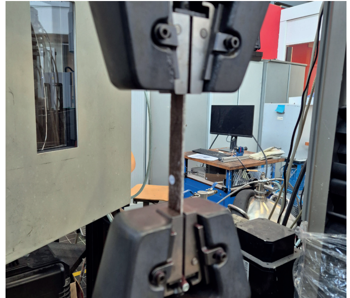
Fig. 7.1 Test set-up tensile test at Mechanical Engineering lab (own image)
