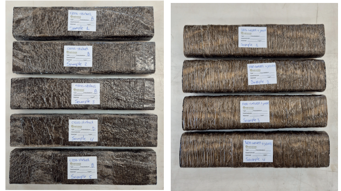
Fig. 7.4 Specimens prepared for 3-point bending test (left: specimen 1-5, right: specimen 6-9) (own image)
