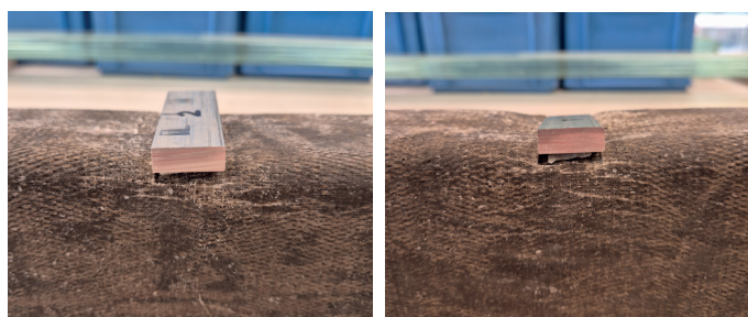
Fig. 8.22 Tested specimens after three-point bending (left: Specimen 11, right: Specimen 12) (own image)
