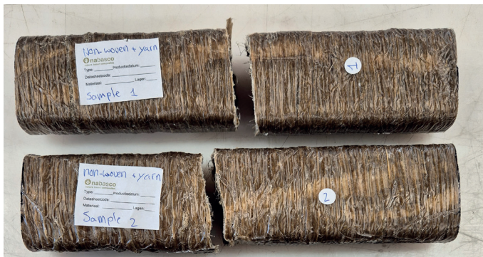
Fig. 7.15 Fractured specimens on bending strength at mse lab (own image)
