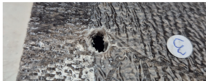
Fig. 7.16 Results profile fixation capacity test: axial loading conditions (own image).
