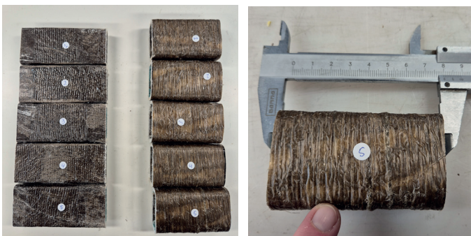
Fig. 7.7 Prepared and measuring specimens for thermal expansion test (own image)
