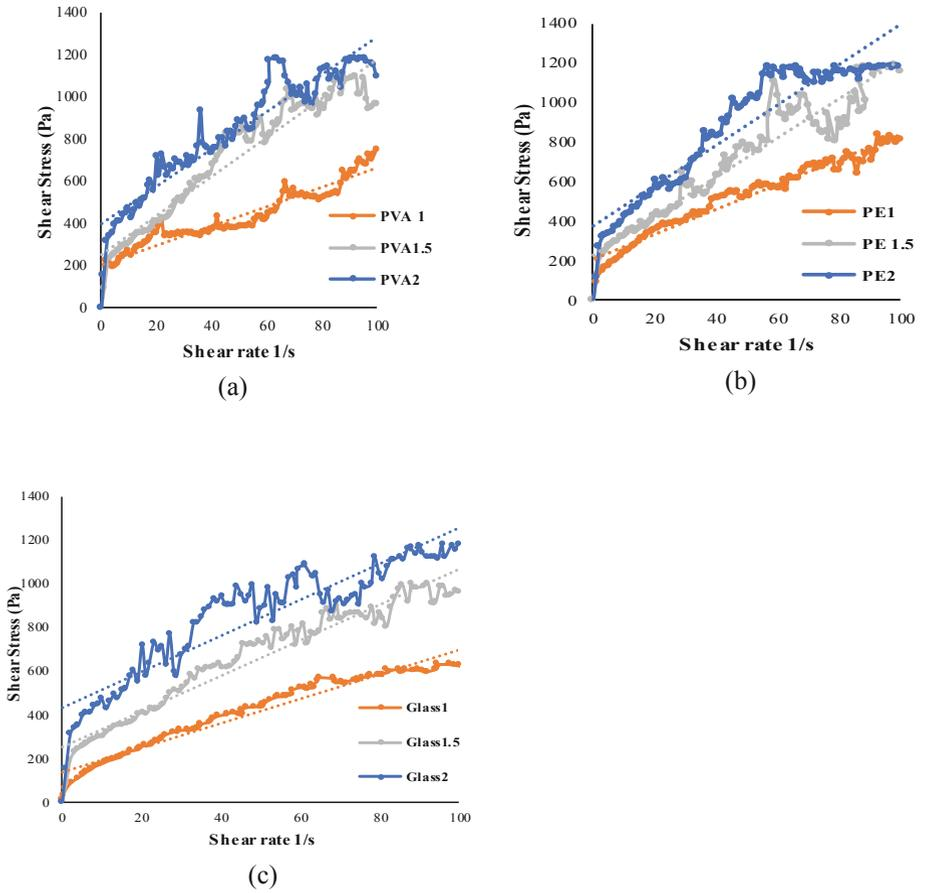
**Fig. 3.** a. Shear stress-shear rate curves for PVA fibres b. Shear stress-shear rate curves for PE fibres c. Shear stress-shear rate curves for glass fibres
