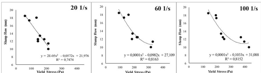
**Fig. 4.** Relationship between yield value and flow spread at different shear rates
