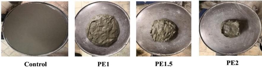
**Fig. 1.** Effect of HDPE fibre addition on the flow spread
