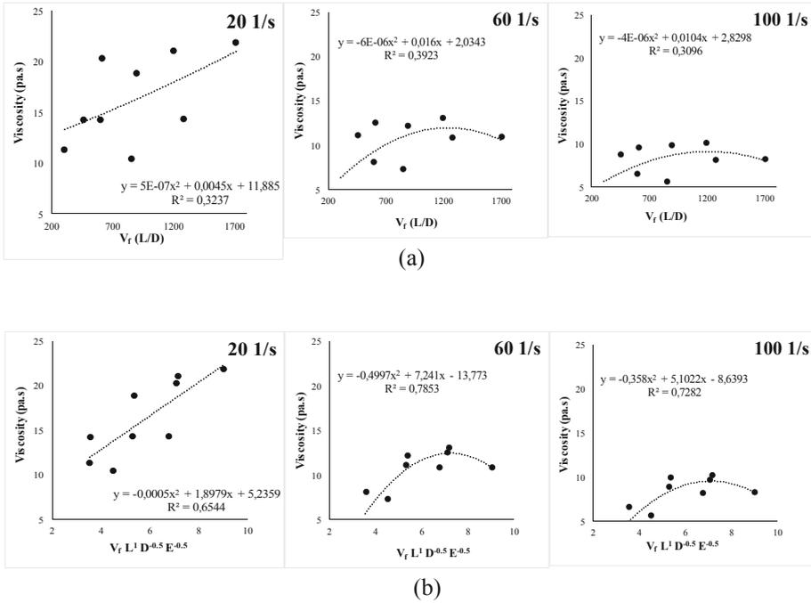
**Fig. 5.** a. Relationship between viscosity and fibre factor b. Relationship between viscosity and modified fibre influence factor
