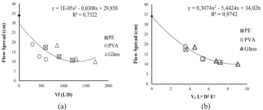
**Fig. 2.** a. Traditional fibre factor b. Modified fibre influence factor
