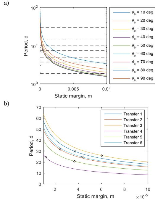
Fig. 14 Oscillation period varying the static margin, for a square  $100 \times 100$  m<sup>2</sup> sail. a) For a range of oscillating amplitudes and oscillating periods. b) For the optimised transfers. Circles represent the design points for achieving the required period on each transfer.
