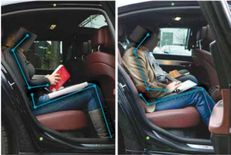
Figure 3.3 Example of body angles observed from the side for reading a book (left) and gaming on tablet (right)
