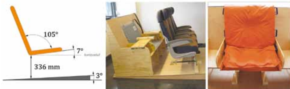
Figure 5.5 Research seat, from left to right: dimensions; complete construction with row of seats in front and inclined floor; free-formable mattress
