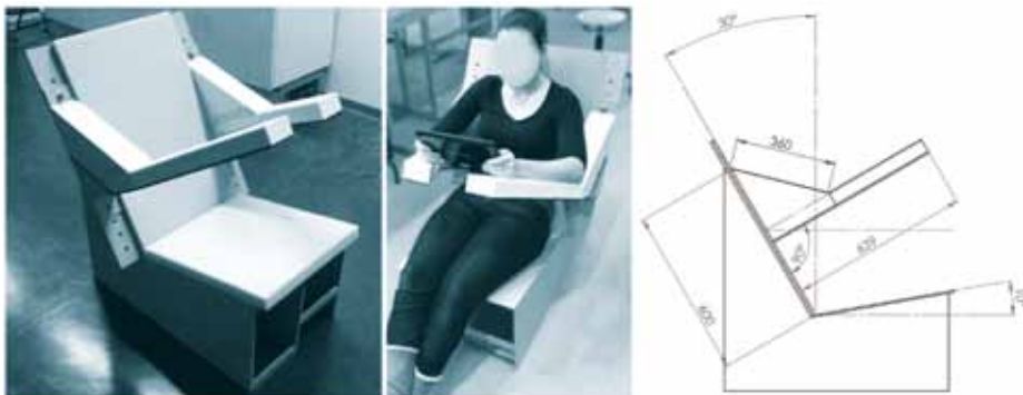
Figure 7.2 Pictures of the mock-up model of the seat (left) and dimensions (mm) of the model with armrests positioned in the second slot from above (right).
