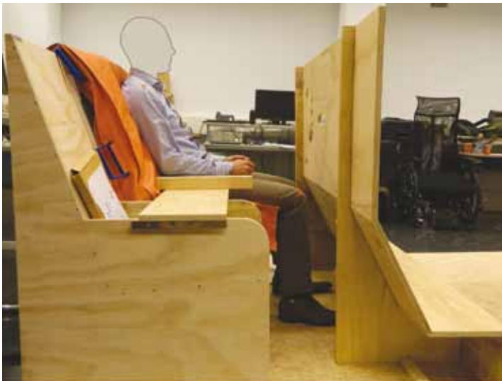
Figure 7.7 Experimental seat: basic wooden frame with vacuum mattress (orange) and seat row in front to simulate restricted legroom
