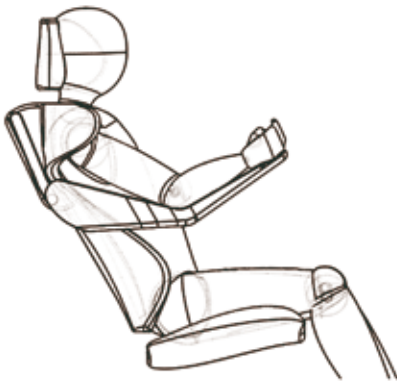
Figure 7.1 Design of the innovative armrests to support mobile device use (design and illustration by Sigrid van Veen)
