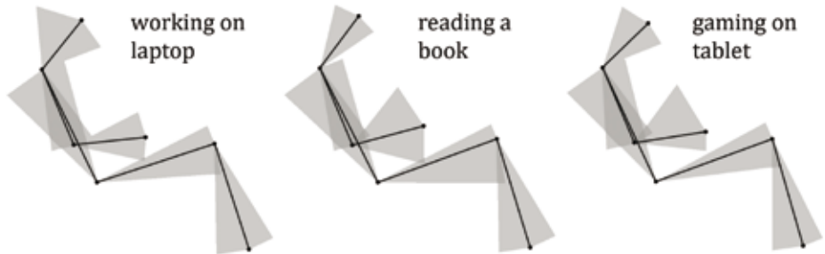
Figure 3.4 Observed body angles observed from the side for three activities; black lines are mean values for each task, grey areas indicate the variation between minimum and maximum angle.
