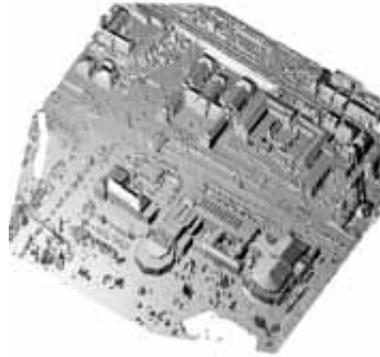
Figure 2.2: Shaded relief made from a point cloud
