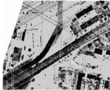
Once all profiles have been segmented they are overlaid. Line segments that have points in common are linked. This linking is continued until surface segments are obtained. As can be seen objects like buildings are conspicuous by the fact that they contain many raised and high line segments.
