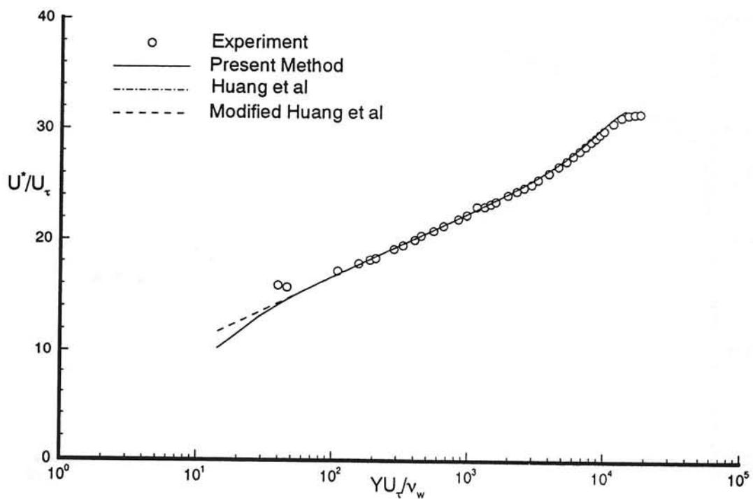
Fig. 21a Transformed velocity profile in semi-logarithmic coordinates. Experimental data from Winter & Gaudet<sup>13</sup>,  $M_\infty = 1.4003$ ,  $Re_\infty = 60234$ , profile 12.
