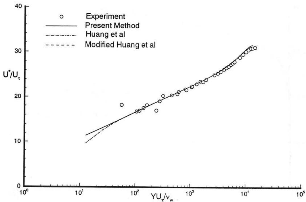
Fig. 8a Transformed velocity profile in semi-logarithmic coordinates. Experimental data from Gaudet<sup>14</sup>,  $M_b = 0.7824$ ,  $Re_0 = 42939$ , profile 2.
