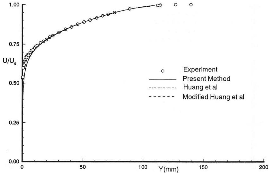
Fig. 30b Untransformed velocity profile in normal coordinates. Experimental data from Winter & Gaudet<sup>13</sup>,  $M_\infty = 2.1865$ ,  $Re_\delta = 14640$ , profile 18.
