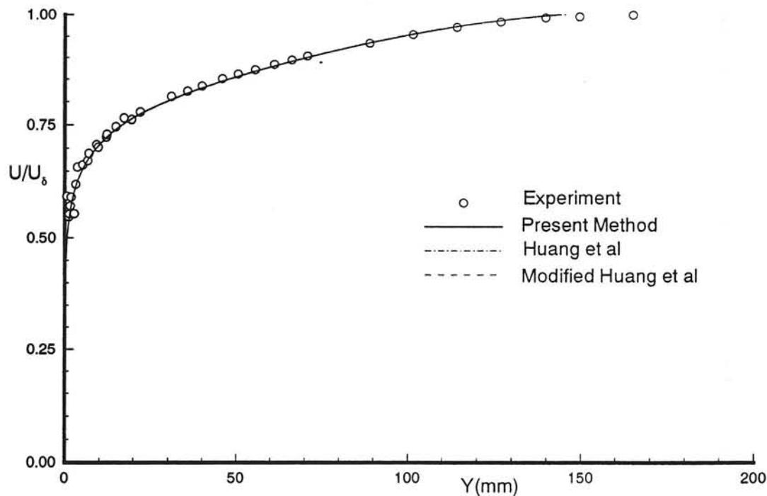
Fig. 8b Untransformed velocity profile in normal coordinates. Experimental data from Gaudet<sup>14</sup>,  $M_\delta = 0.7824$ ,  $Re_\delta = 42939$ , profile 2.
