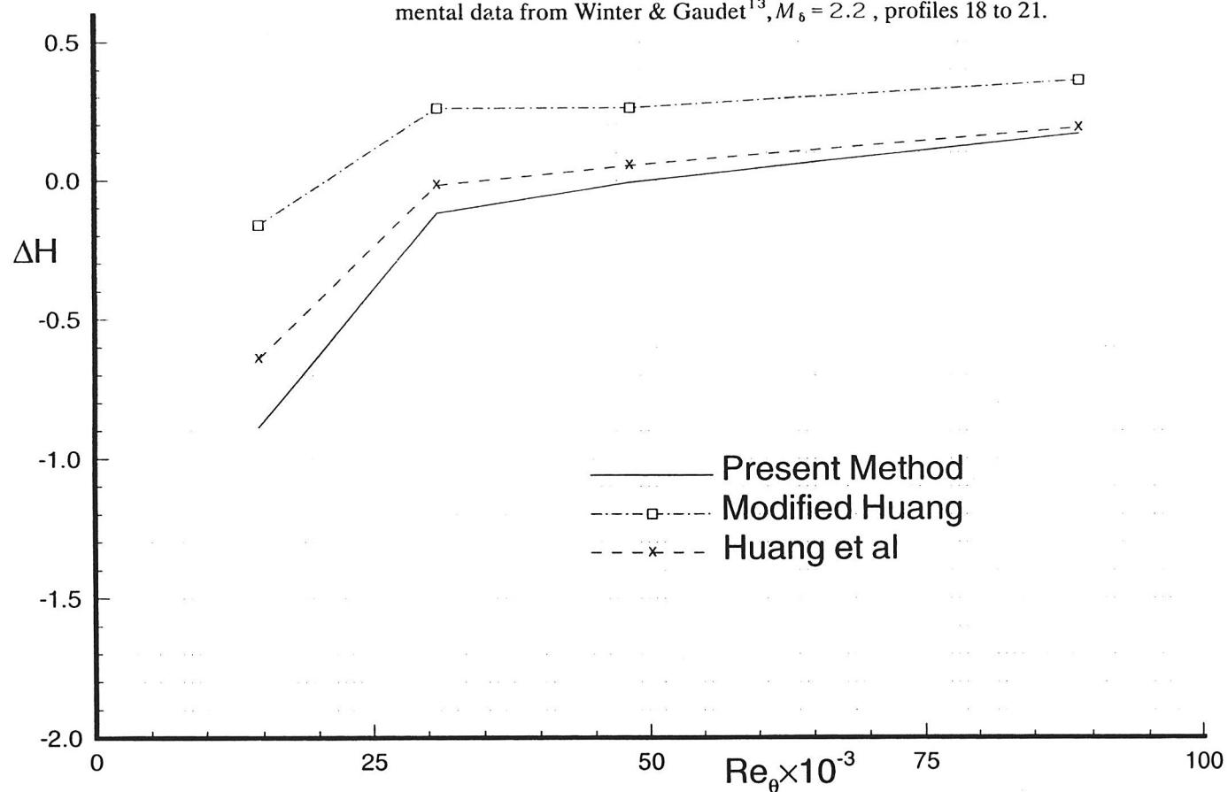
Fig. 43 Percent error in shape parameter  $\Delta H = (1 - H_{cal}/H_{exp}) \times 100\%$ . Experimental data from Winter & Gaudet<sup>13</sup>,  $M_b = 2.2$ , profiles 39 to 48.
