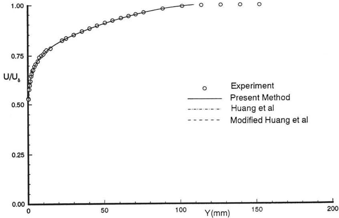
Fig. 23b Untransformed velocity profile in normal coordinates. Experimental data from Winter & Gaudet<sup>13</sup>,  $M_\delta = 1.4003$ ,  $Re_\delta = 128035$ , profile 14.
