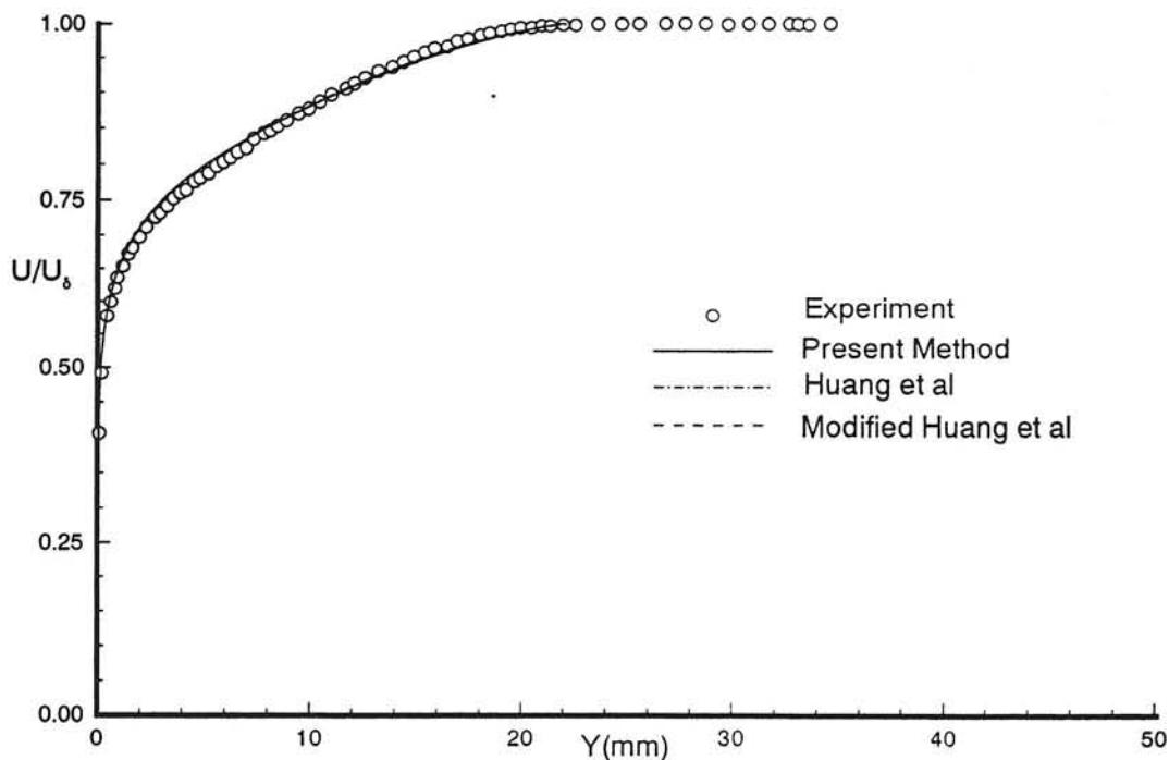
Fig. 10b Untransformed velocity profile in normal coordinates. Experimental data from Collins et al<sup>15</sup>,  $M_\delta = 0.9664$ ,  $Re_\delta = 18650$ , profile JPL-A-91.
