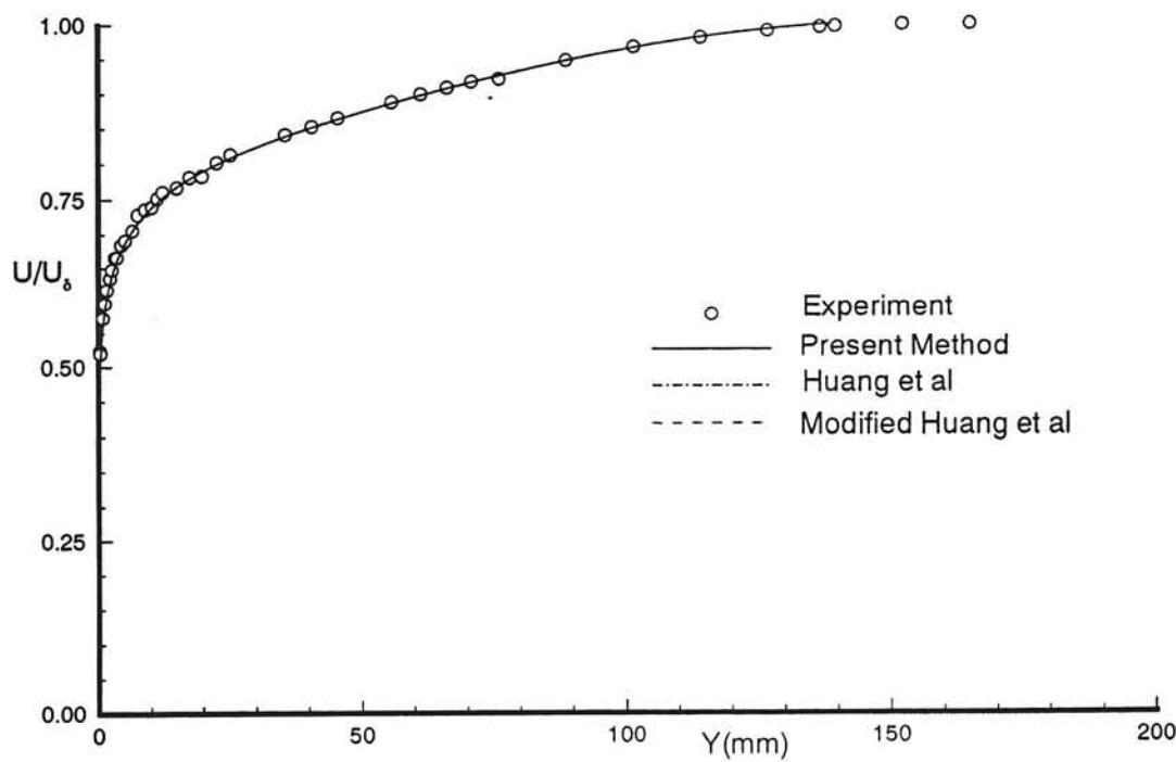
Fig. 13b Untransformed velocity profile in normal coordinates. Experimental data from Winter & Gaudet<sup>13</sup>,  $M_\delta = 0.7933$ ,  $Re_\delta = 157450$ , profile 9.
