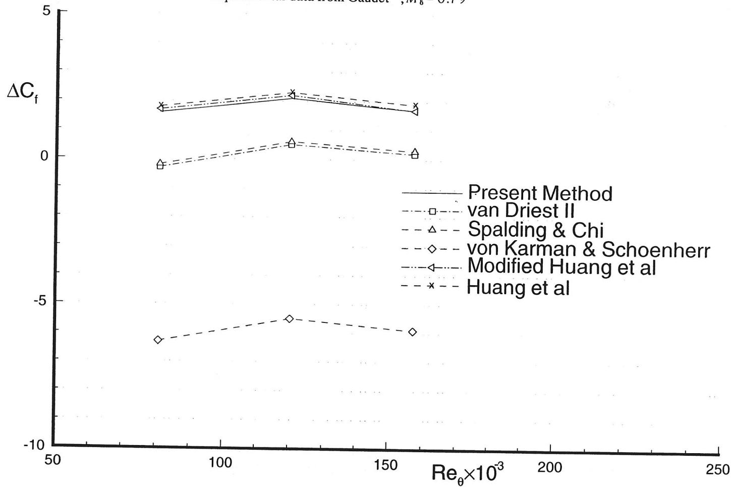
Fig. 4 Percent error in skin friction coefficient  $\Delta C_f = (1 - C_{f, \text{cal}}/C_{f, \text{exp}}) \times 100\%$ .
