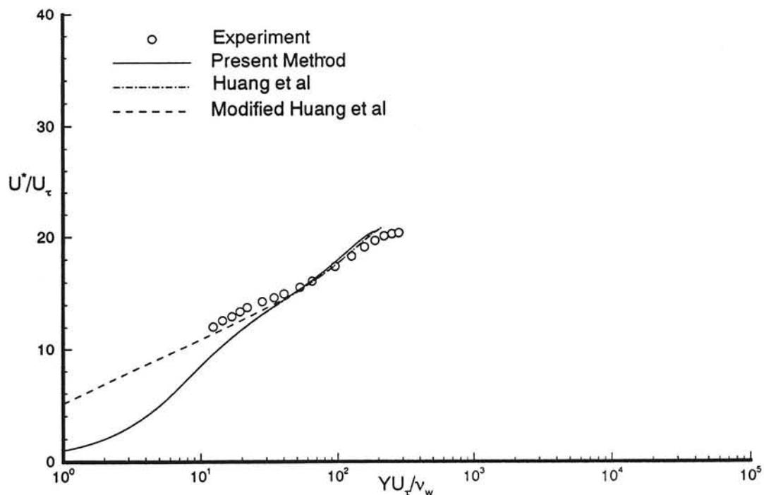
Fig. 27a Transformed velocity profile in semi-logarithmic coordinates. Experimental data from Stalmach<sup>23</sup>,  $M_\delta = 3.6840$ ,  $Re_\delta = 2115.3$ , case 58020301.
