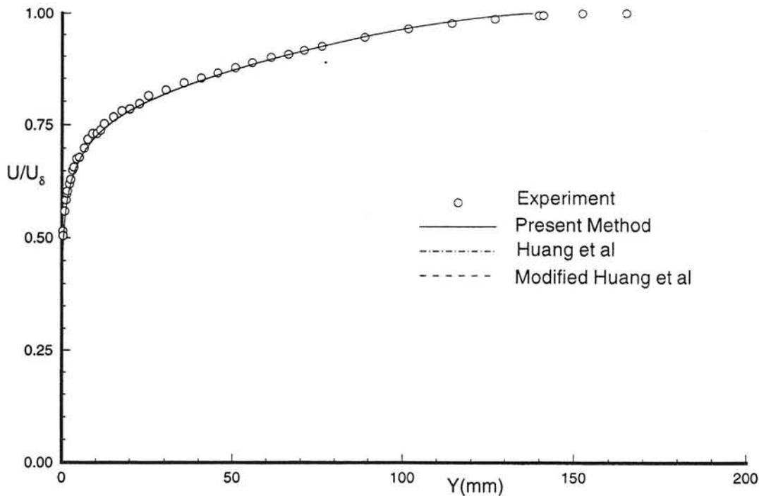
Fig. 11b Untransformed velocity profile in normal coordinates. Experimental data from Winter & Gaudet<sup>13</sup>,  $M_\delta = 0.7904$ ,  $Re_\delta = 81000$ , profile 7.
