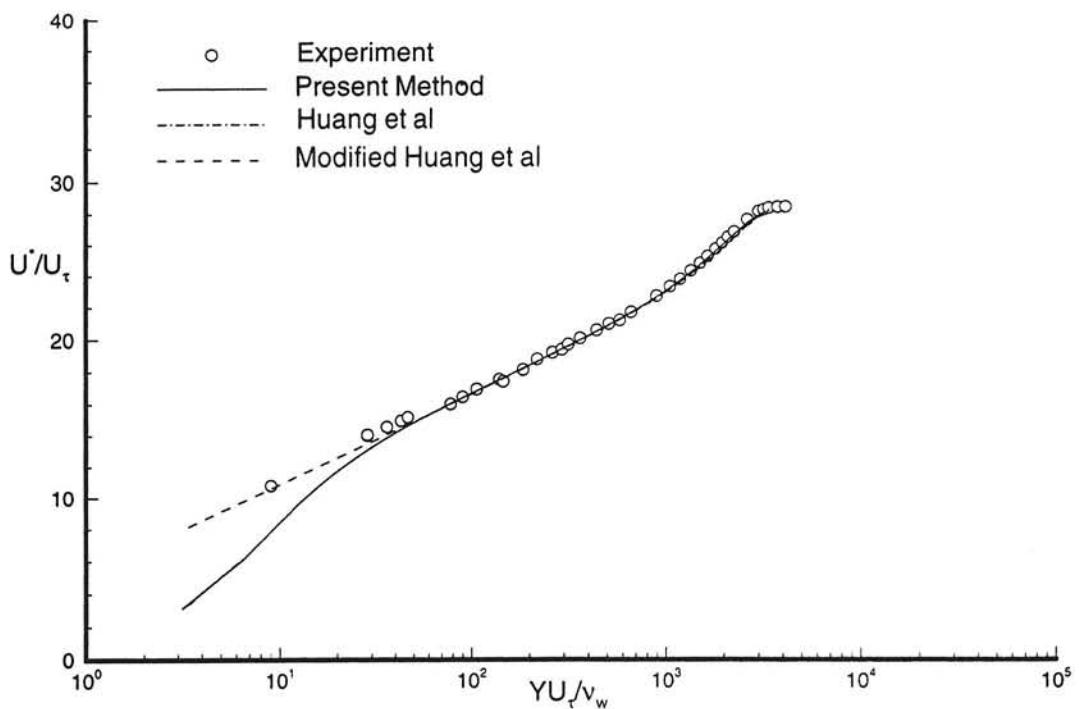
Fig. 32a Transformed velocity profile in semi-logarithmic coordinates. Experimental data from Winter & Gaudet <sup>13</sup>,  $M_\infty = 2.1984$ ,  $Re_0 = 19939$ , profile 39.
