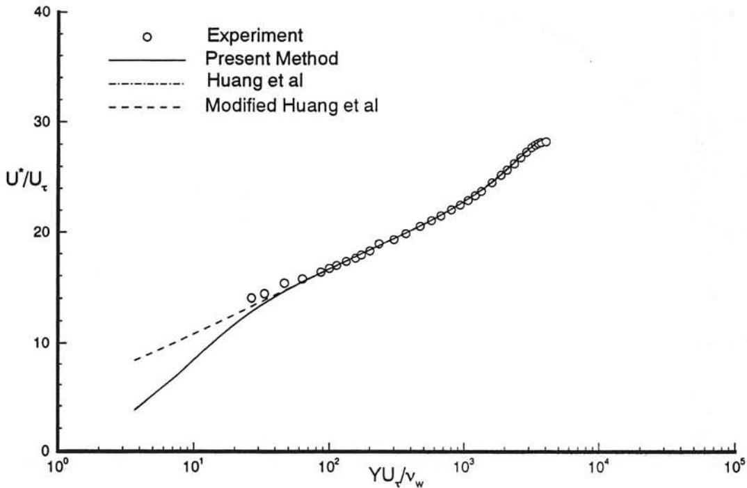
Fig. 17a Transformed velocity profile in semi-logarithmic coordinates. Experimental data from Morkovin & Phinney<sup>24</sup>,  $M_\delta = 1.770$ ,  $Re_\theta = 17672$ , case 58060101.
