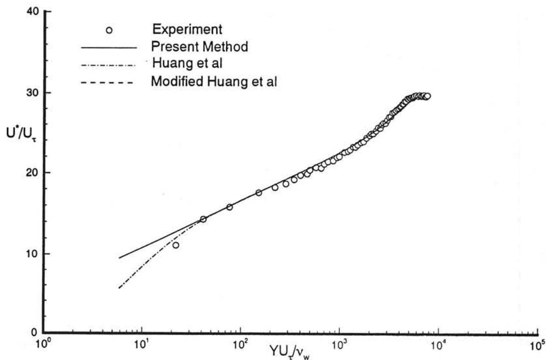
Fig. 9a Transformed velocity profile in semi-logarithmic coordinates. Experimental data from Collins et al<sup>15</sup>,  $M_\infty = 0.5927$ ,  $Re_\theta = 18870$ , profile JPL-A-51.
