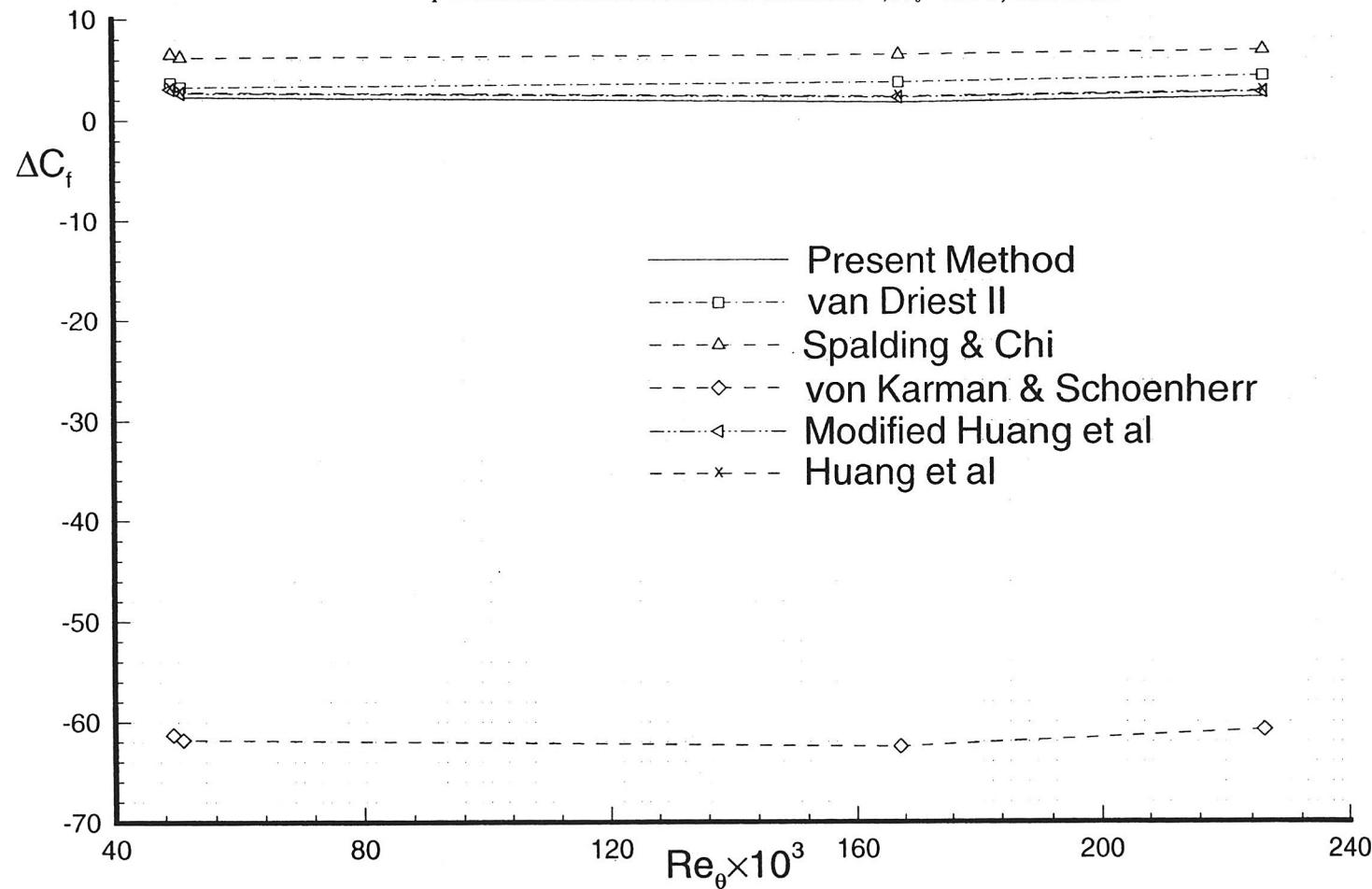
Fig. 26 Percent error in skin friction coefficient  $\Delta C_f = (1 - C_{f,cal}/C_{f,exp}) \times 100\%$ .
