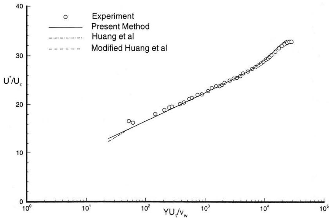
Fig. 11a Transformed velocity profile in semi-logarithmic coordinates. Experimental data from Winter & Gaudet<sup>13</sup>,  $M_\infty = 0.7904$ ,  $Re_\theta = 81000$ , profile 7.
