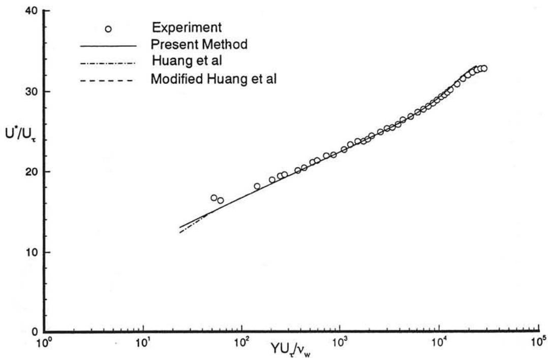
Fig. 7a Transformed velocity profile in semi-logarithmic coordinates. Experimental data from Winter & Gaudet<sup>13</sup>,  $M_\infty = 0.20$ ,  $Re_\infty = 55982$ , profile 1.
