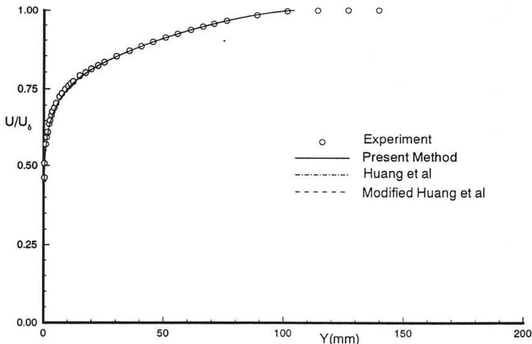
Fig. 18b Untransformed velocity profile in normal coordinates. Experimental data from Winter & Gaudet<sup>13</sup>,  $M_\delta = 1.5970$ ,  $R\delta_0 = 56479$ , profile 16.
