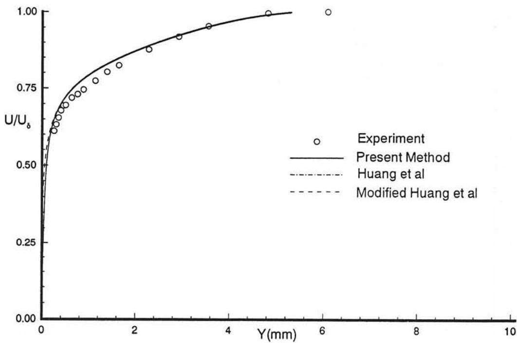
Fig. 29b Untransformed velocity profile in normal coordinates. Experimental data from Stalmach<sup>23</sup>,  $M_\delta = 3.681$ ,  $Re_\delta = 10484$ , case 58020306.
