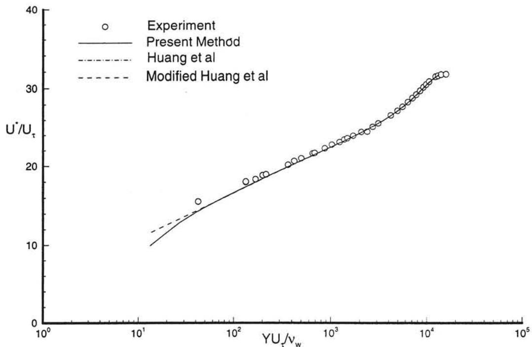
Fig. 33a Transformed velocity profile in semi-logarithmic coordinates. Experimental data from Winter & Gaudet <sup>13</sup>,  $M_\delta = 2.2082$ ,  $Re_\delta = 84259$ , profile 48.
