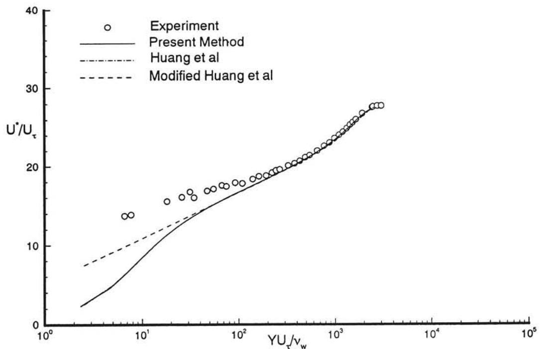
Fig. 30a Transformed velocity profile in semi-logarithmic coordinates. Experimental data from Winter & Gaudet<sup>13</sup>,  $M_\infty = 2.1865$ ,  $Re_\infty = 14640$ , profile 18.
