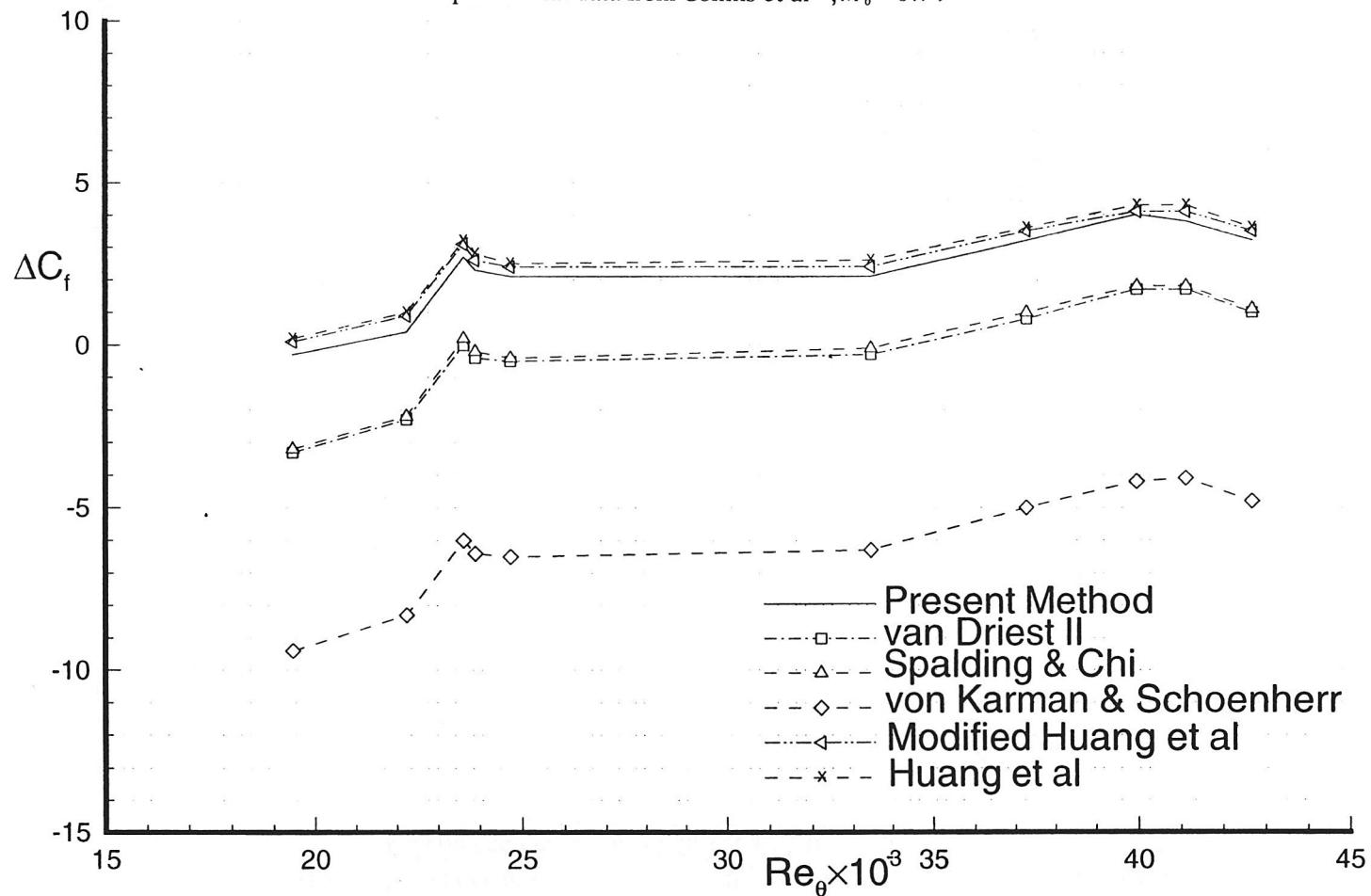
Fig. 6 Percent error in skin friction coefficient  $\Delta C_f = (1 - C_{f, \text{cal}}/C_{f, \text{exp}}) \times 100\%$ .
