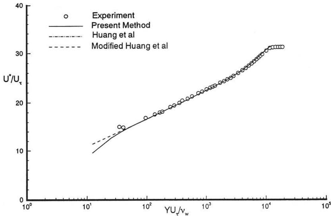
Fig. 16a Transformed velocity profile in semi-logarithmic coordinates. Experimental data from Winter & Gaudet<sup>13</sup>,  $M_\infty = 1.5970$ ,  $Re_0 = 56479$ , profile 15.
