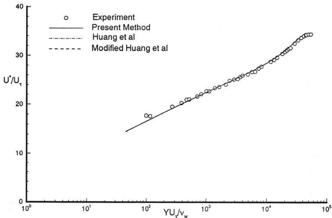
Fig. 13a Transformed velocity profile in semi-logarithmic coordinates. Experimental data from Winter & Gaudet<sup>13</sup>,  $M_\infty = 0.7933$ ,  $Rho_0 = 157450$ , profile 9.
