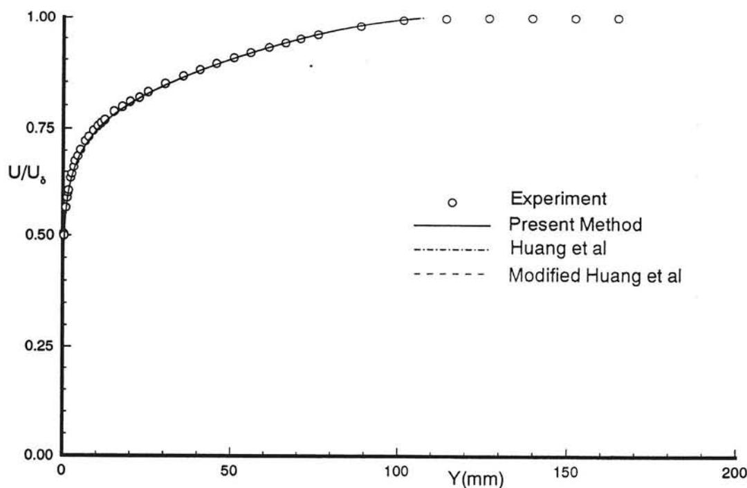
Fig. 16b Untransformed velocity profile in normal coordinates. Experimental data from Winter & Gaudet<sup>13</sup>,  $M_\delta = 1.5970$ ,  $Re_0 = 56479$ , profile 15.
