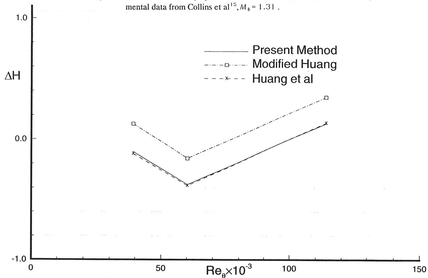
Fig. 42 Percent error in shape parameter  $\Delta H = (1 - H_{cal}/H_{exp}) \times 100\%$ . Experimental data from Winter & Gaudet<sup>13</sup>,  $M_6 = 2.2$ , profiles 18 to 21.
