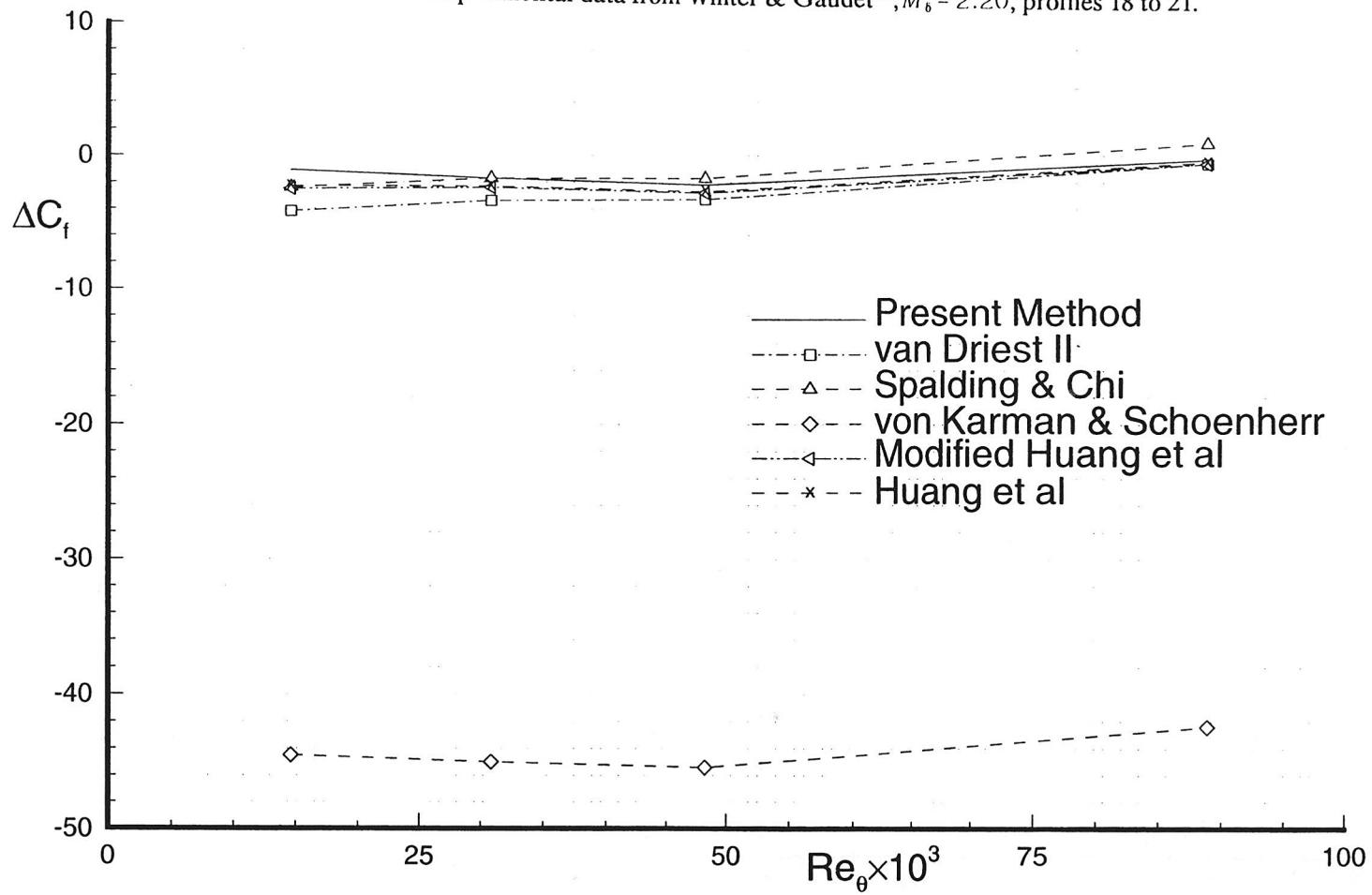
Fig. 25 Percent error in skin friction coefficient  $\Delta C_f = (1 - C_{f,cal}/C_{f,exp}) \times 100\%$ .
