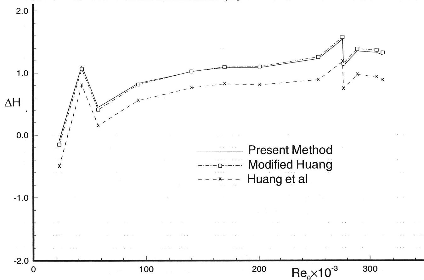
Fig. 40 Percent error in shape parameter  $\Delta H = (1 - H_{cal}/H_{exp}) \times 100\%$ . Experimental data from Collins et al<sup>15</sup>,  $M_\infty = 1.31$ .
