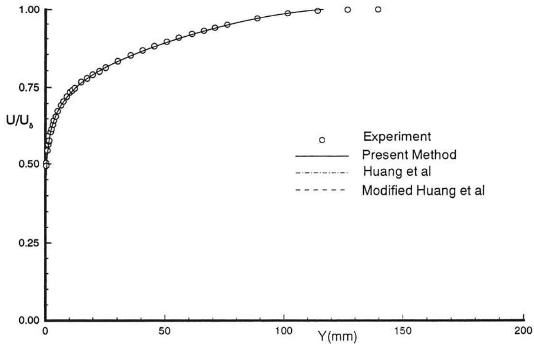
Fig. 20b Untransformed velocity profile in normal coordinates. Experimental data from Winter & Gaudet<sup>13</sup>,  $M_\delta = 1.3951$ ,  $Re_\delta = 39333$ , profile 11.
