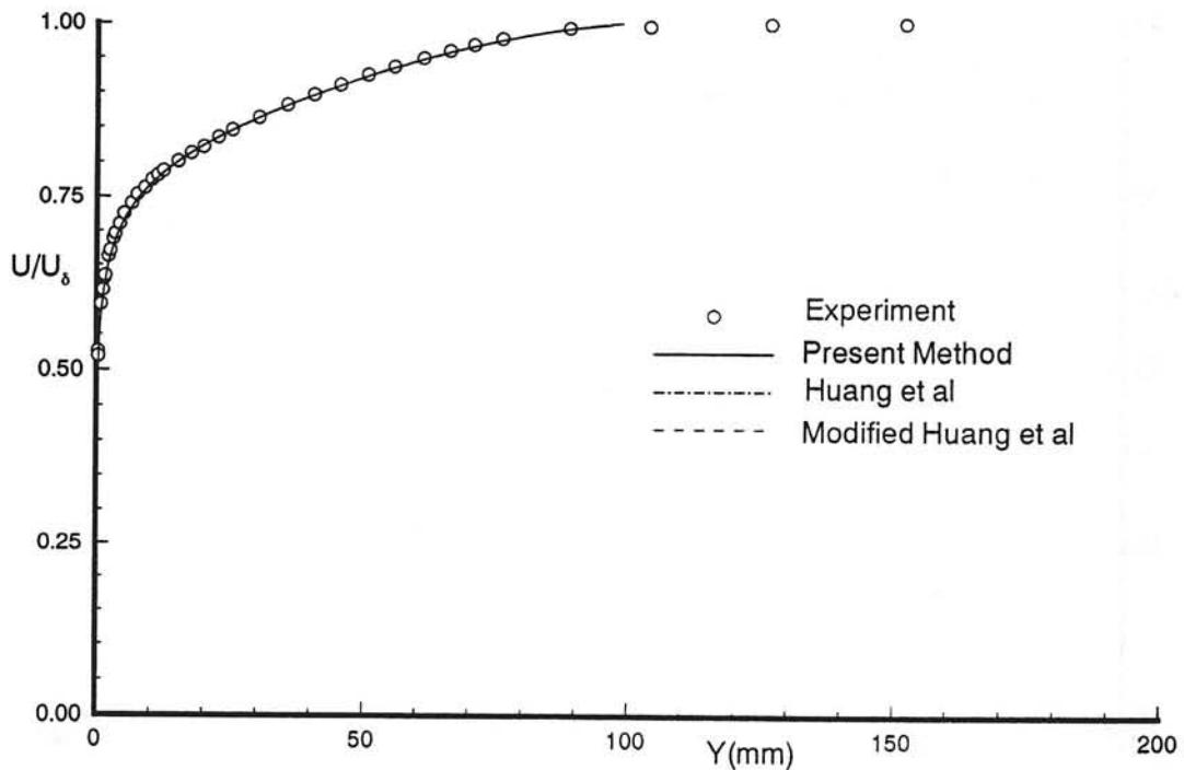
Fig. 31b Untransformed velocity profile in normal coordinates. Experimental data from Winter & Gaudet<sup>13</sup>,  $M_\infty = 2.2064$ ,  $R\delta_0 = 88907$ , profile 21.
