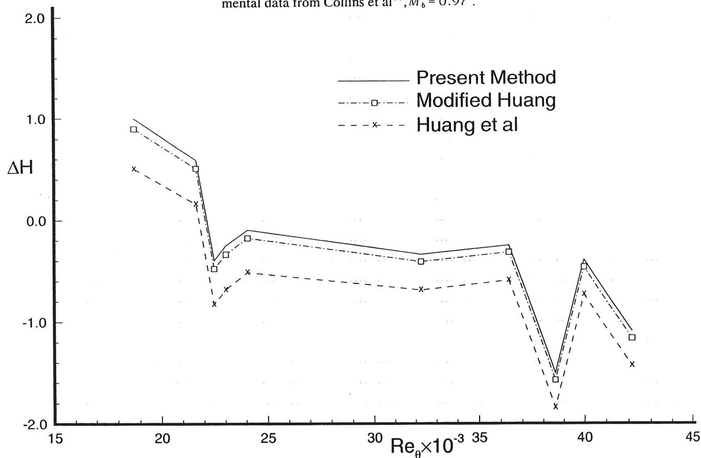
Fig. 37 Percent error in shape parameter  $\Delta H = (1 - H_{cal}/H_{exp}) \times 100\%$ . Experimental data from Winter & Gaudet<sup>13</sup>,  $M_6 = 0.20$ .
