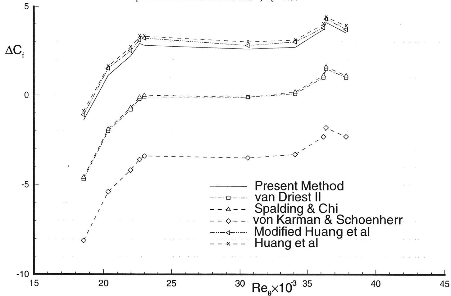
Fig. 5 Percent error in skin friction coefficient  $\Delta C_f = (1 - C_{f, \text{cal}}/C_{f, \text{exp}}) \times 100\%$ .
