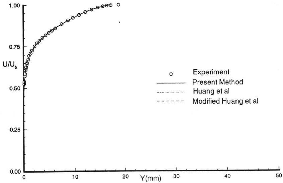
Fig. 17b Untransformed velocity profile in normal coordinates. Experimental data from Morkovin<sup>24</sup>,  $M_\delta = 1.770$ ,  $Re_\delta = 17672$ , case 58060101.
