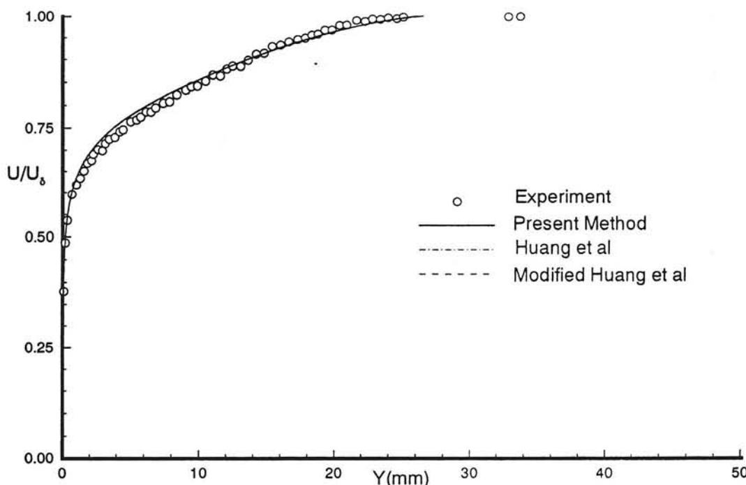
Fig. 9b Untransformed velocity profile in normal coordinates. Experimental data from Collins et al<sup>15</sup>,  $M_\delta = 0.5927$ ,  $Re_\delta = 18870$ , profile JPL-A-51.
