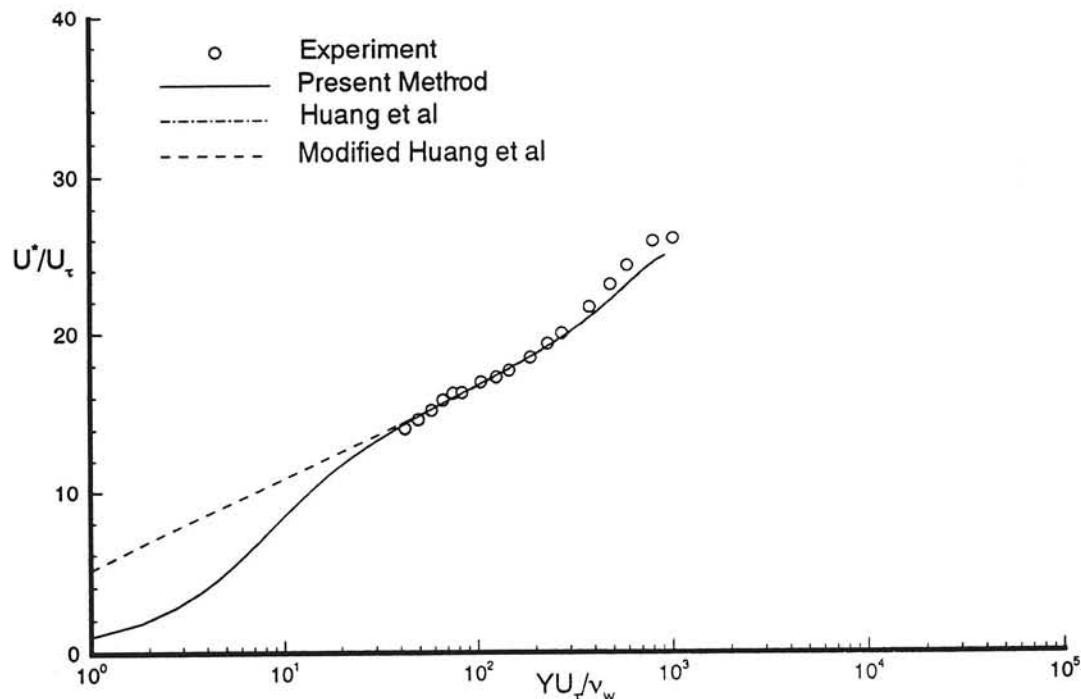
Fig. 29a Transformed velocity profile in semi-logarithmic coordinates. Experimental data from Stalmach<sup>23</sup>,  $M_\infty = 3.681$ ,  $Re_\infty = 10484$ , case 58020306.
