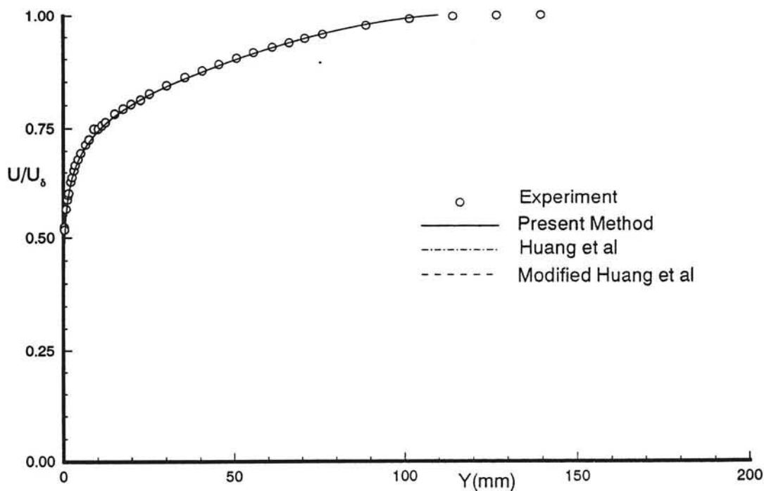
Fig. 21b Untransformed velocity profile in normal coordinates. Experimental data from Winter & Gaudet<sup>13</sup>,  $M_b = 1.4003$ ,  $R\alpha_0 = 60234$ , profile 12.
