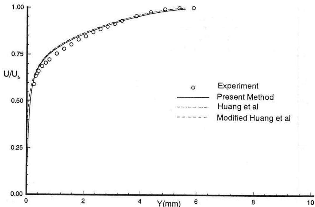
Fig. 28b Untransformed velocity profile in normal coordinates. Experimental data from Stalmach<sup>23</sup>,  $M_\delta = 3.6670$ ,  $Re_\delta = 8134.9$ , case 58020304.
