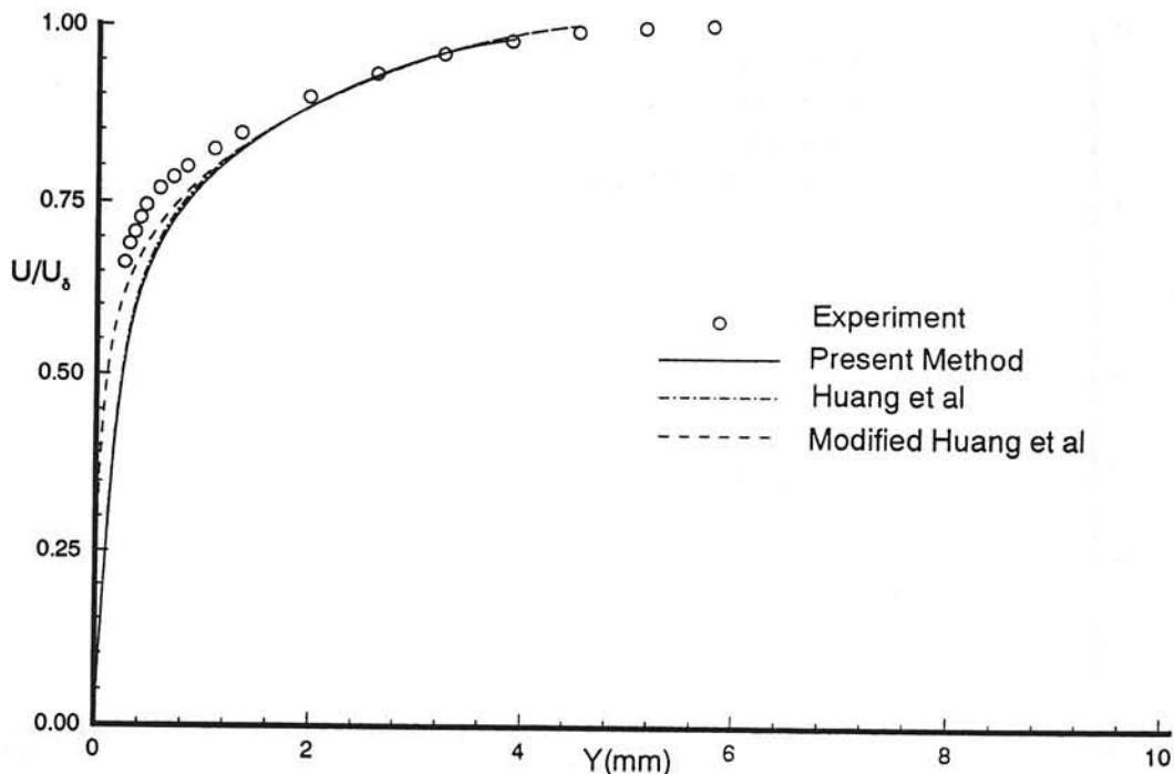
Fig. 27b Untransformed velocity profile in normal coordinates. Experimental data from Stalmach<sup>23</sup>,  $M_\delta = 3.6840$ ,  $Re_\delta = 2115.3$ , case 58020301.
