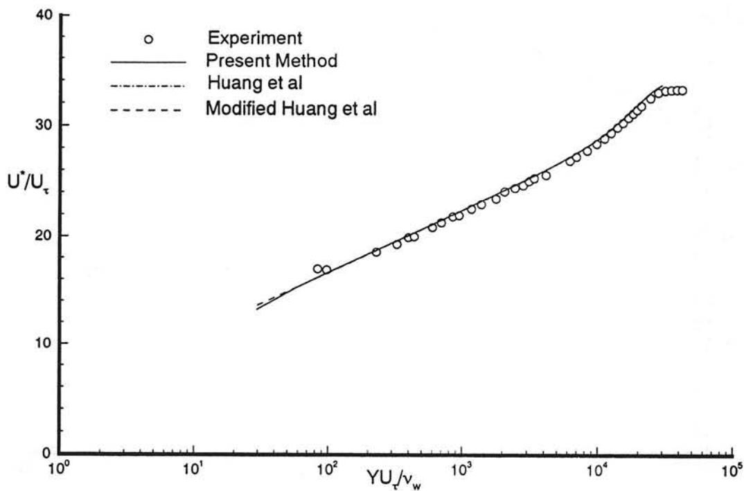
Fig. 23a Transformed velocity profile in semi-logarithmic coordinates. Experimental data from Winter & Gaudet<sup>13</sup>,  $M_b = 1.4003$ ,  $Re_b = 128035$ , profile 14.
