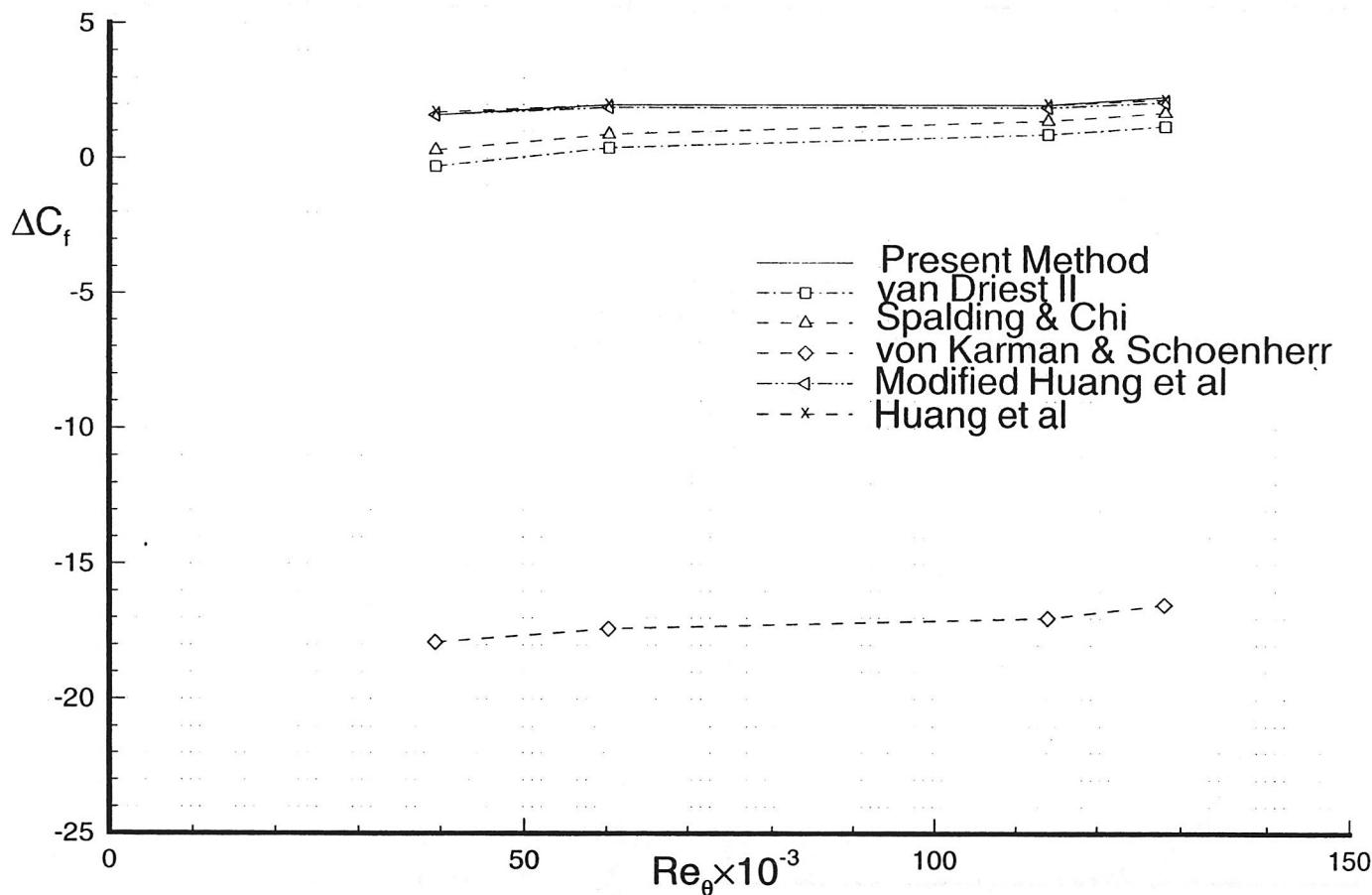
Fig. 15 Percent error in skin friction coefficient  $\Delta C_f = (1 - C_{f,cal}/C_{f,exp}) \times 100\%$ .
