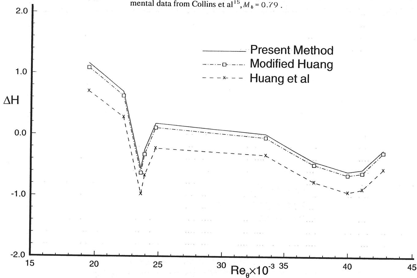
Fig. 36 Percent error in shape parameter  $\Delta H = (1 - H_{\text{cal}}/H_{\text{exp}}) \times 100\%$ . Experimental data from Collins et al<sup>15</sup>,  $M_b = 0.97$ .
