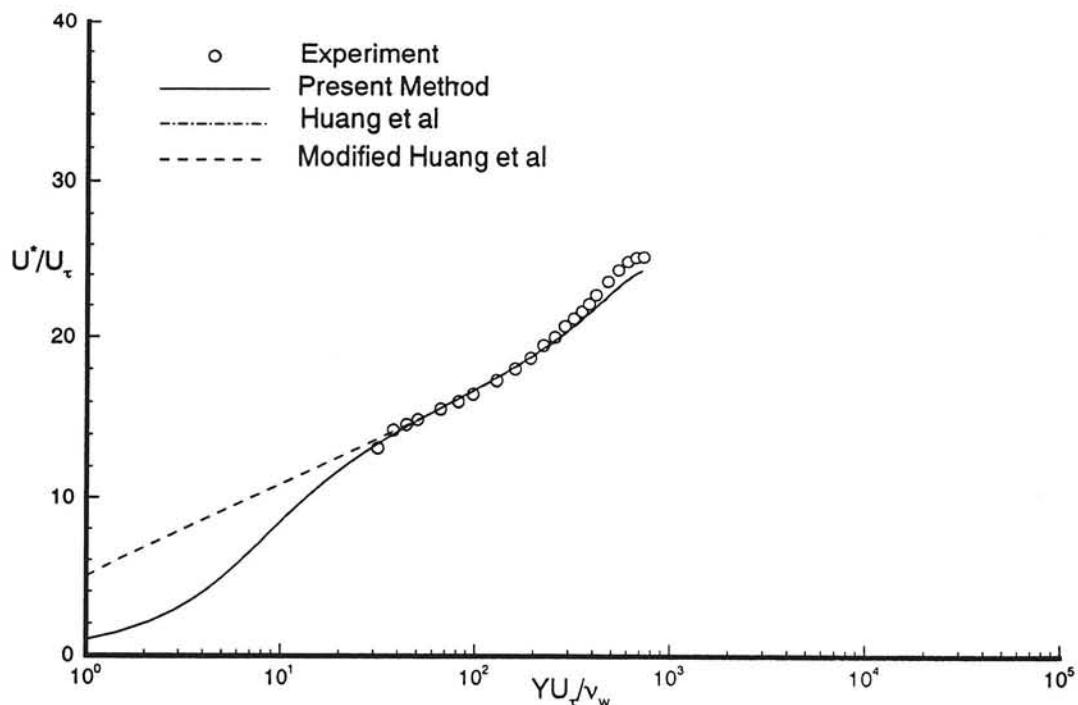
Fig. 28a Transformed velocity profile in semi-logarithmic coordinates. Experimental data from Stalmach<sup>23</sup>,  $M_\infty = 3.6670$ ,  $Re_\infty = 8134.9$ , case 58020304.
