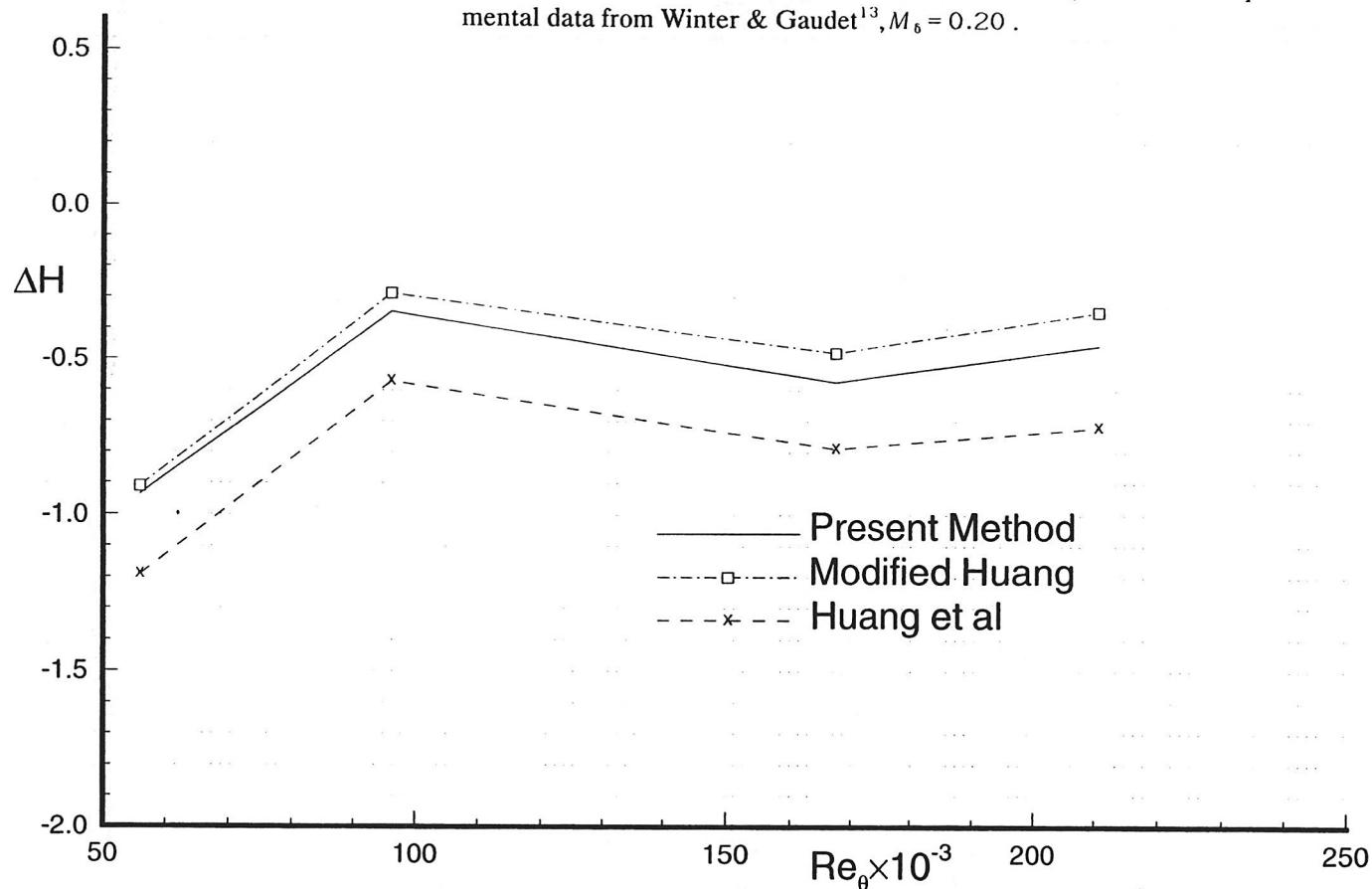
Fig. 38 Percent error in shape parameter  $\Delta H = (1 - H_{cal}/H_{exp}) \times 100\%$ . Experimental data from Winter & Gaudet<sup>13</sup>,  $M_6 = 0.79$ .
