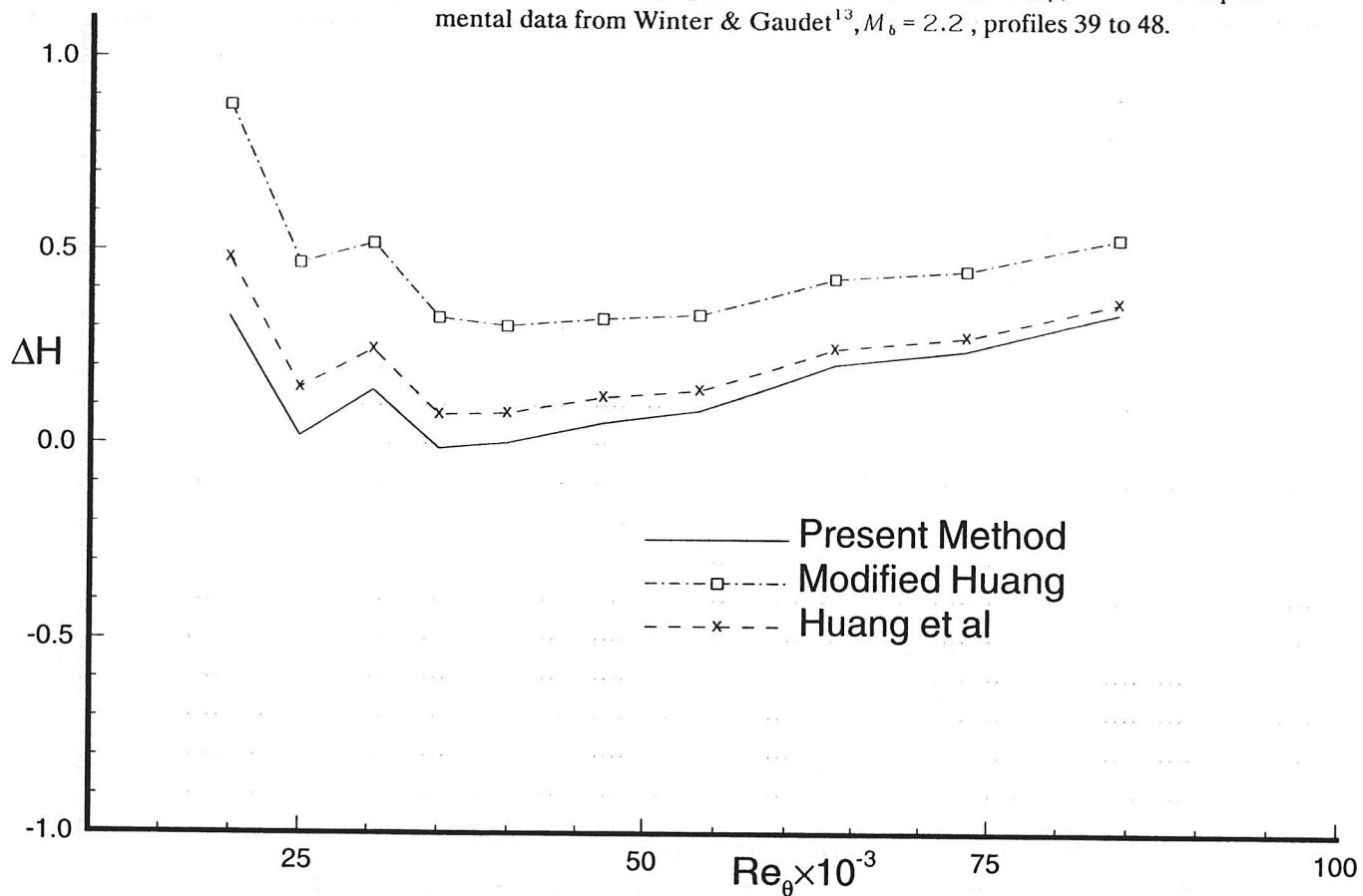
Fig. 44 Percent error in shape parameter  $\Delta H = (1 - H_{cal}/H_{exp}) \times 100\%$ . Experimental data from Moore & Harkness<sup>23</sup>,  $M_\infty = 2.90$ , case 6502.
