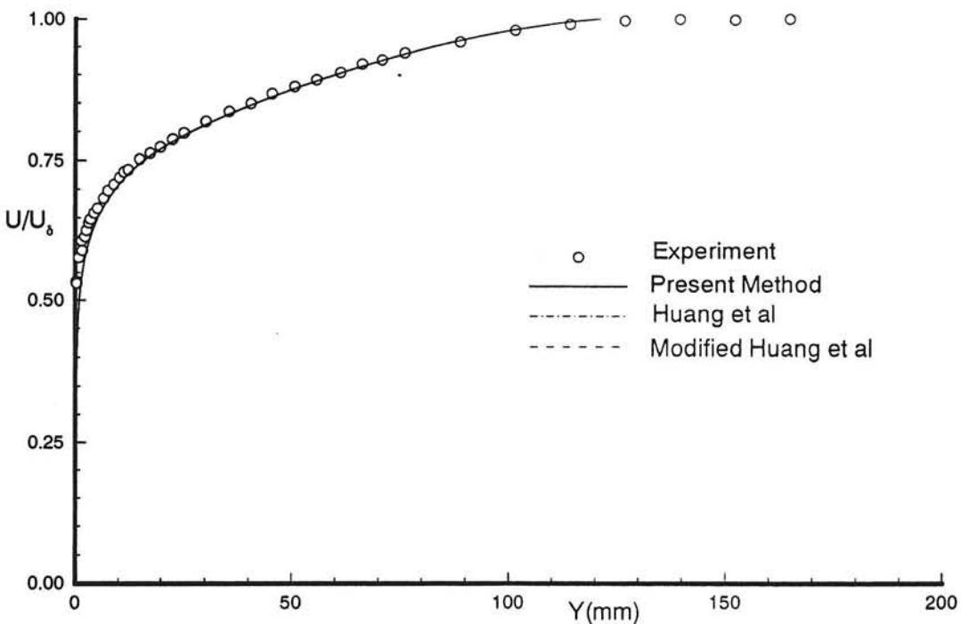
Fig. 19b Untransformed velocity profile in normal coordinates. Experimental data from Winter & Gaudet<sup>13</sup>,  $M_\delta = 1.3943$ ,  $Re_\delta = 17914$ , profile 10.
