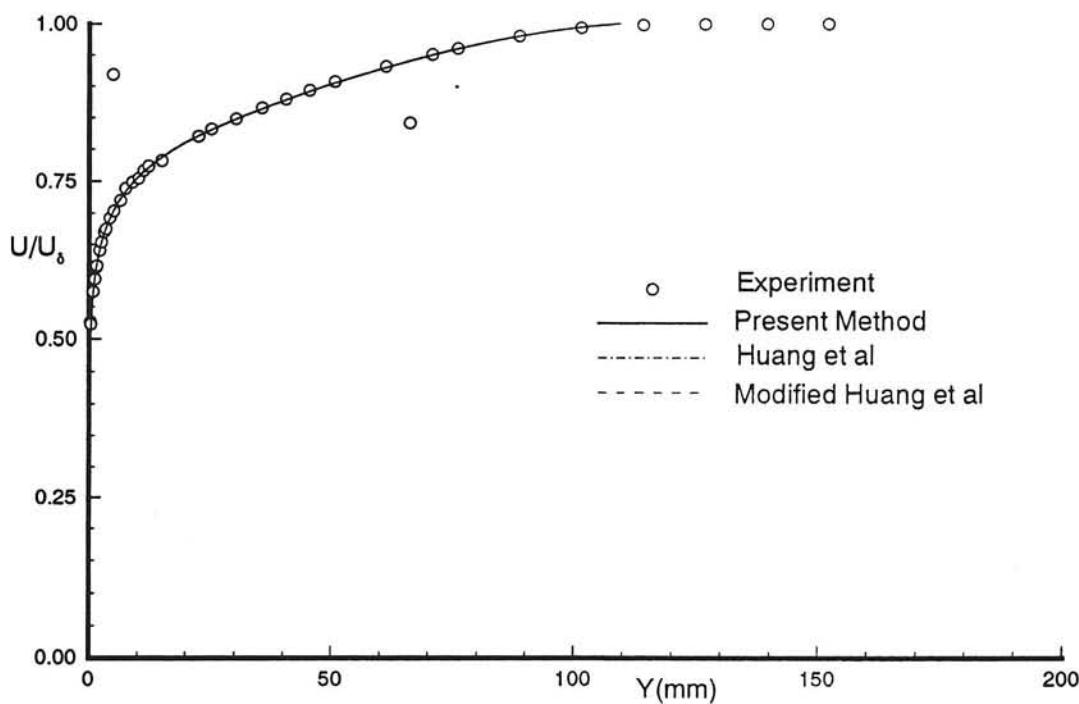
Fig. 22b Untransformed velocity profile in normal coordinates. Experimental data from Winter & Gaudet<sup>13</sup>,  $M_\delta = 1.3999$ ,  $Re_\delta = 113948$ , profile 13.
