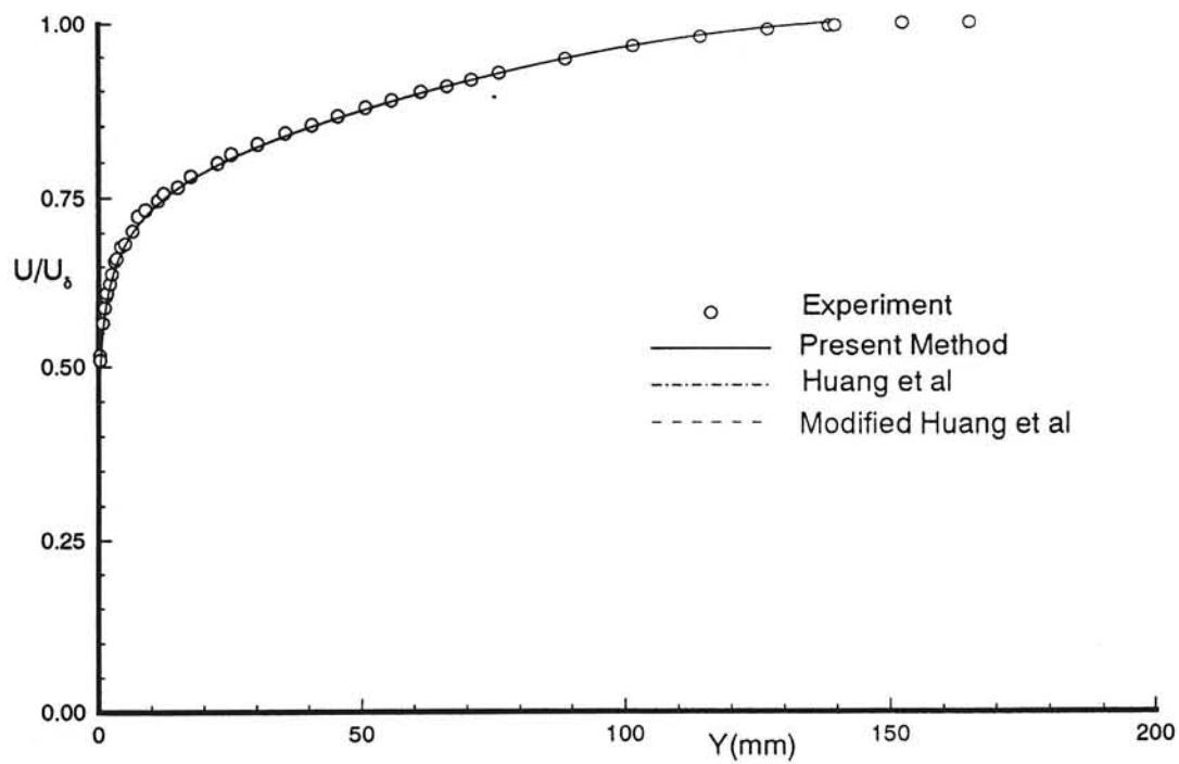
Fig. 12b Untransformed velocity profile in normal coordinates. Experimental data from Winter & Gaudet<sup>13</sup>,  $M_\delta = 0.7930$ ,  $Re_\delta = 120366$ , profile 8.
