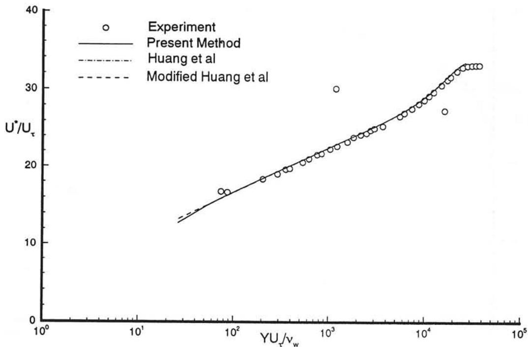
Fig. 22a Transformed velocity profile in semi-logarithmic coordinates. Experimental data from Winter & Gaudet<sup>13</sup>,  $M_\delta = 1.3999$ ,  $Re_\delta = 113948$ , profile 13.
