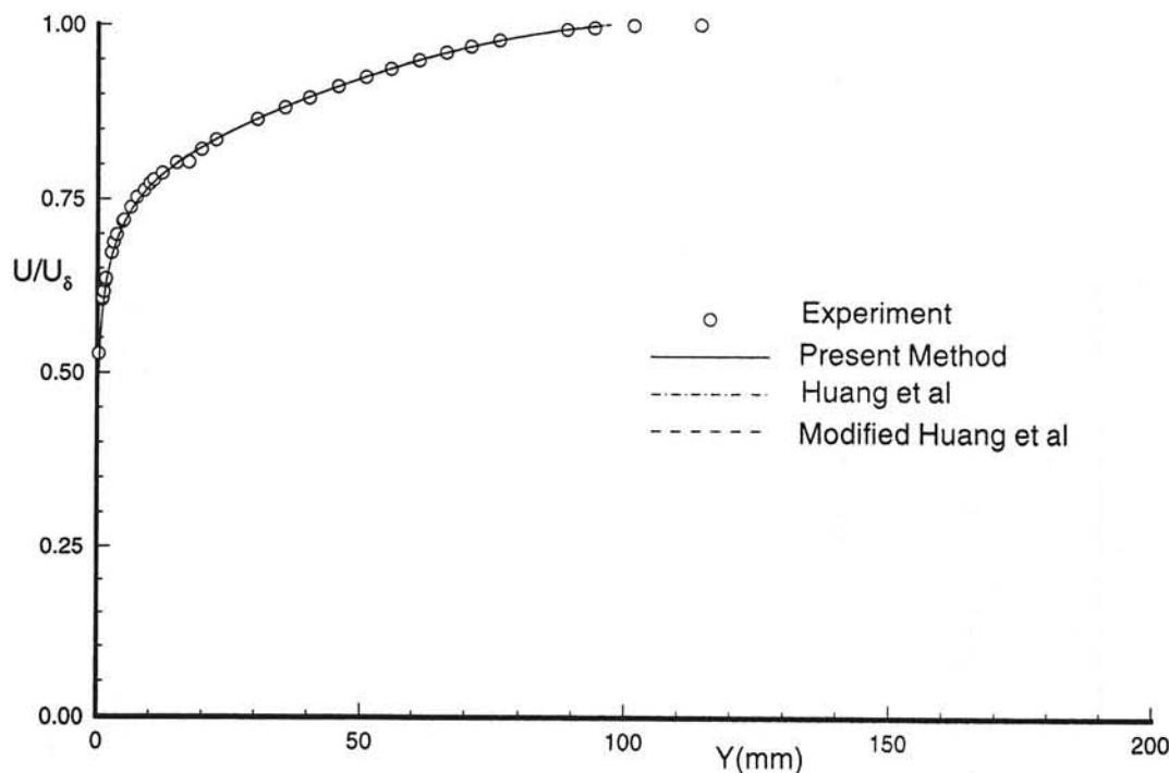
Fig. 33b Untransformed velocity profile in normal coordinates. Experimental data from Winter & Gaudet <sup>13</sup>,  $M_\delta = 2.2082$ ,  $R\delta = 8.1259$ , profile 48.
