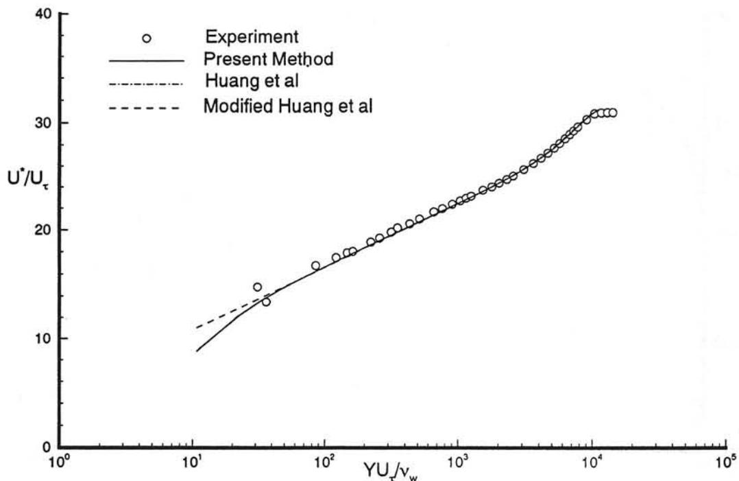
Fig. 18a Transformed velocity profile in semi-logarithmic coordinates. Experimental data from Winter & Gaudet<sup>13</sup>,  $M_\infty = 1.8002$ ,  $Re_\delta = 53671$ , profile 16.
