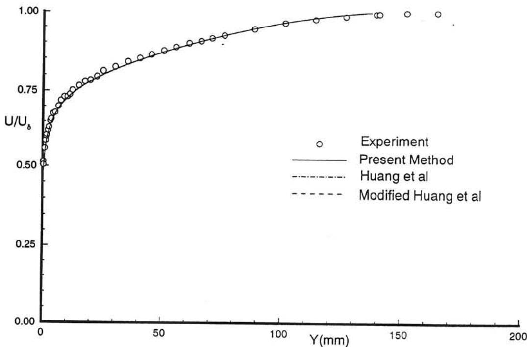
Fig. 7b Untransformed velocity profile in normal coordinates. Experimental data from Winter & Gaudet<sup>13</sup>,  $M_\delta = 0.20$ ,  $R\alpha_0 = 55982$ , profile 1.
