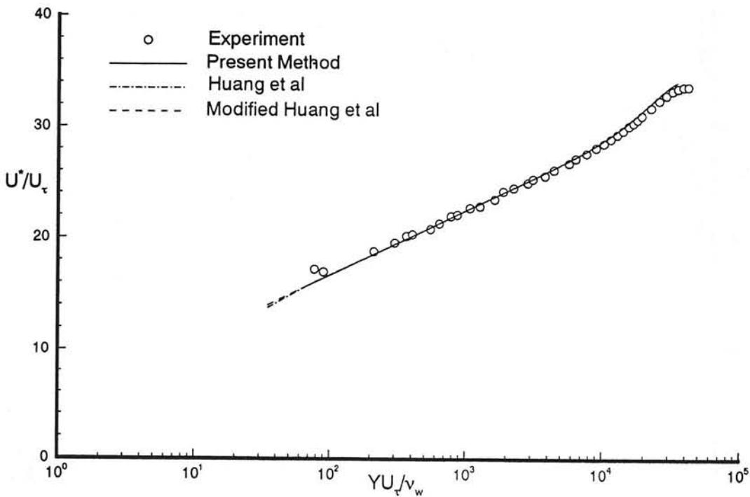
Fig. 12a Transformed velocity profile in semi-logarithmic coordinates. Experimental data from Winter & Gaudet<sup>13</sup>,  $M_\delta = 0.7930$ ,  $Re_\delta = 120366$ , profile 8.
