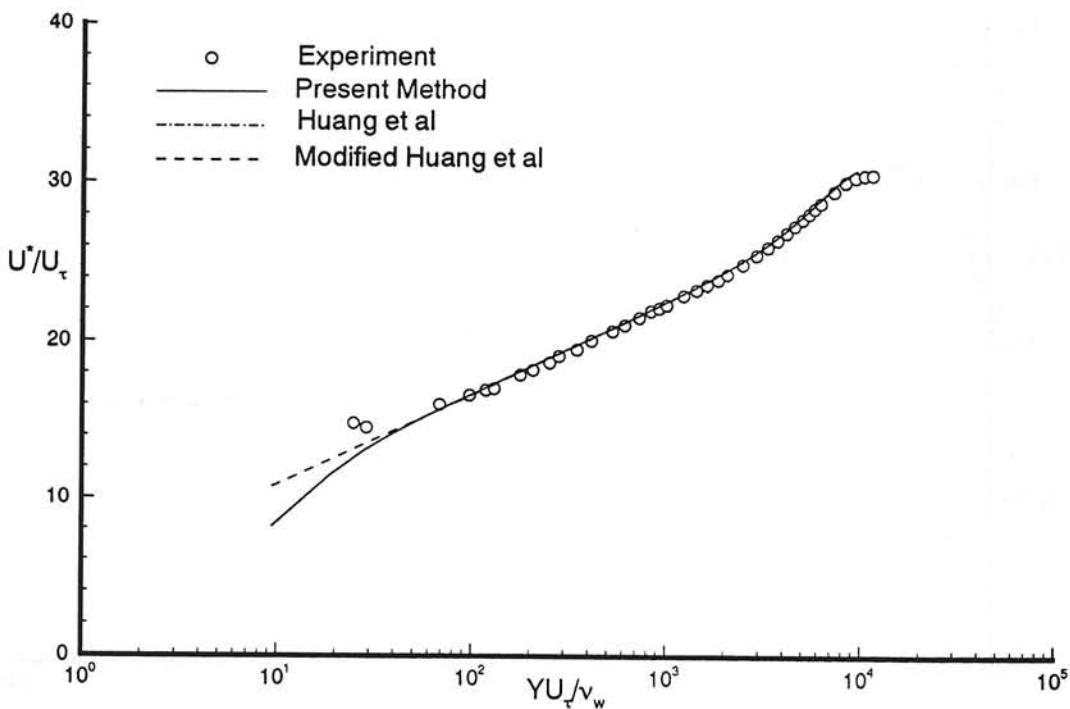
Fig. 20a Transformed velocity profile in semi-logarithmic coordinates. Experimental data from Winter & Gaudet<sup>13</sup>,  $M_\infty = 1.3951$ ,  $Re_\infty = 39333$ , profile 11.
