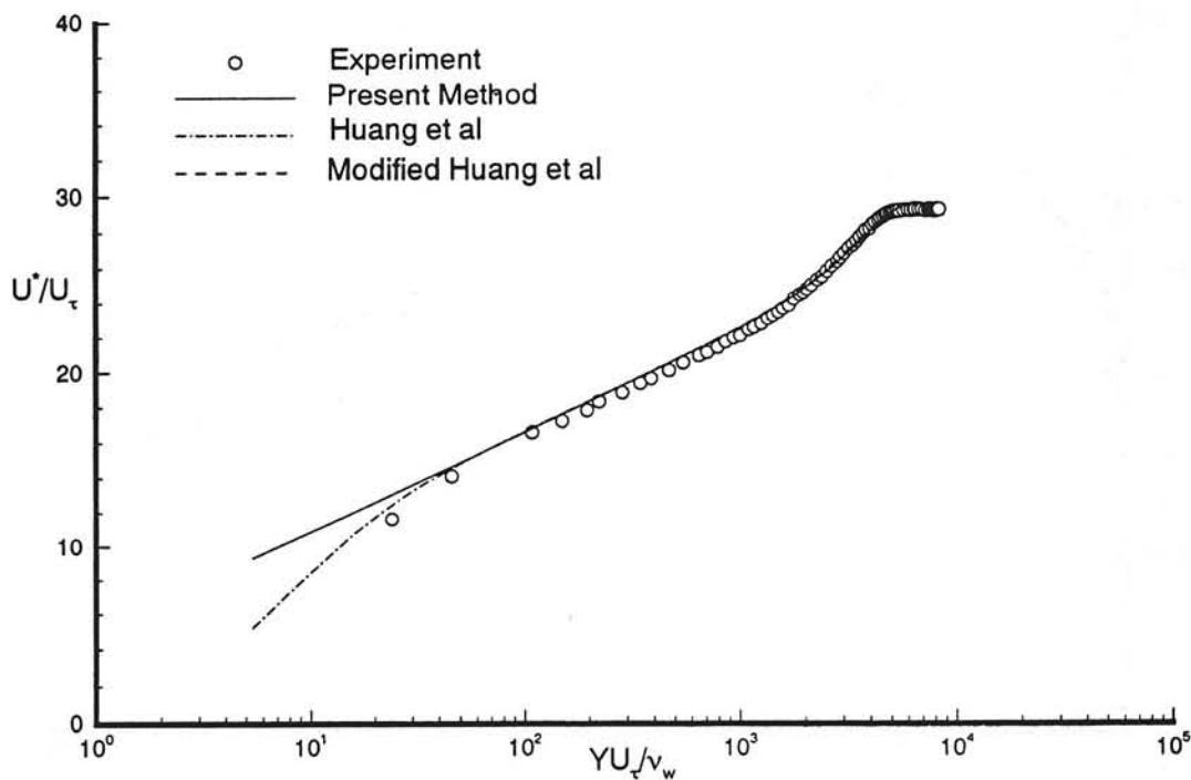
Fig. 10a Transformed velocity profile in semi-logarithmic coordinates. Experimental data from Collins et al<sup>15</sup>,  $M_\infty = 0.9664$ ,  $Re_\infty = 18650$ , profile JPL-A-91.
