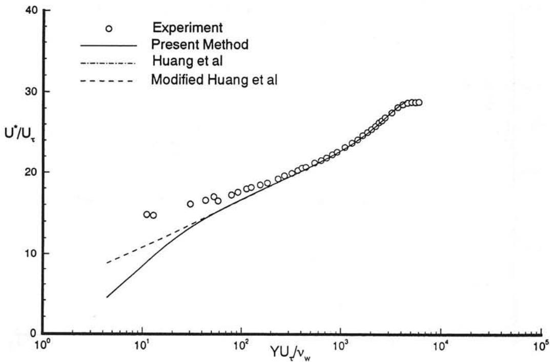
Fig. 19a Transformed velocity profile in semi-logarithmic coordinates. Experimental data from Winter & Gaudet<sup>13</sup>,  $M_\infty = 1.3943$ ,  $Re_0 = 17914$ , profile 10.
