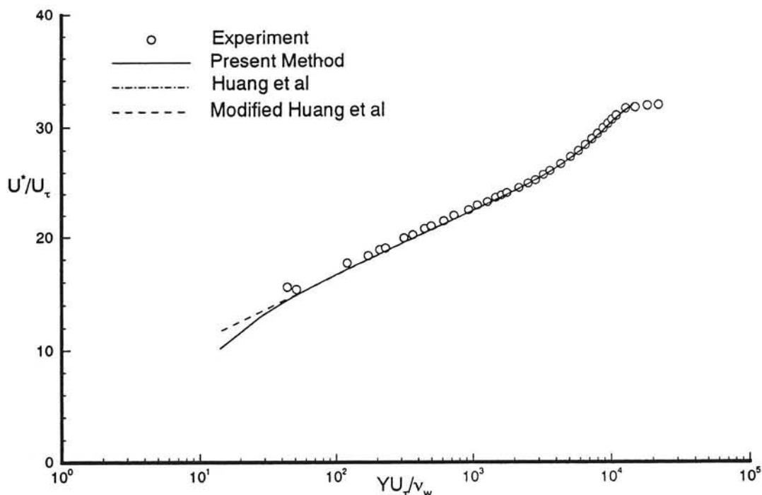
Fig. 31a Transformed velocity profile in semi-logarithmic coordinates. Experimental data from Winter & Gaudet<sup>13</sup>,  $M_\infty = 2.2064$ ,  $Re_\theta = 88907$ , profile 21.
