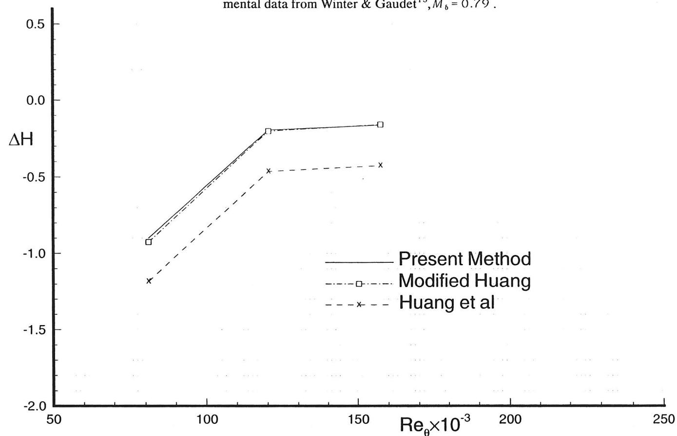
Fig. 39 Percent error in shape parameter  $\Delta H = (1 - H_{cal}/H_{exp}) \times 100\%$ . Experimental data from Gaudet<sup>13</sup>,  $M_\infty = 0.784$ .
