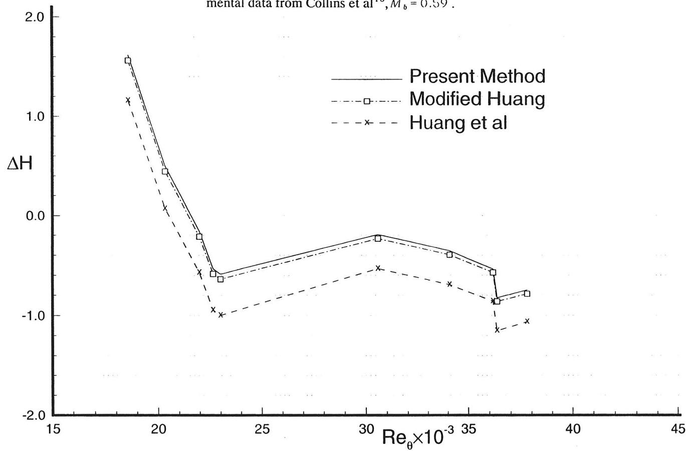
Fig. 35 Percent error in shape parameter  $\Delta H = (1 - H_{cal}/H_{exp}) \times 100\%$ . Experimental data from Collins et al<sup>15</sup>,  $M_b = 0.79$ .
