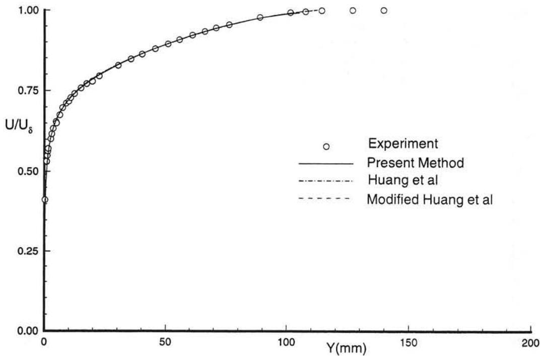
Fig. 32b Untransformed velocity profile in normal coordinates. Experimental data from Winter & Gaudet <sup>13</sup>,  $M_\infty = 2.1984$ ,  $Re_\infty = 19939$ , profile 39.
