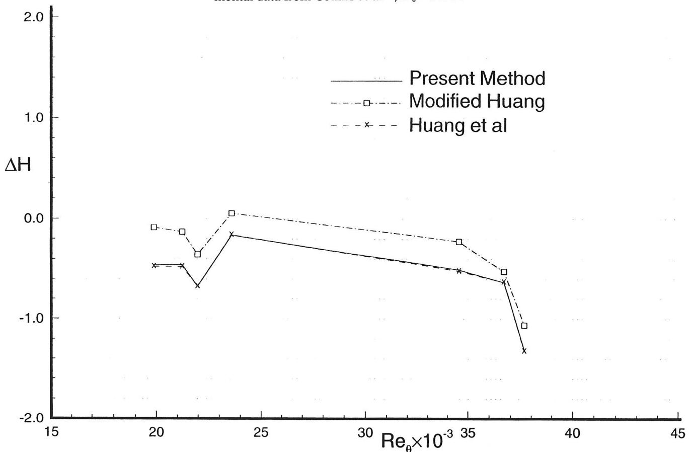
Fig. 41 Percent error in shape parameter  $\Delta H = (1 - H_{cal}/H_{exp}) \times 100\%$ . Experimental data from Collins et al<sup>15</sup>,  $M_\infty = 1.31$ .
