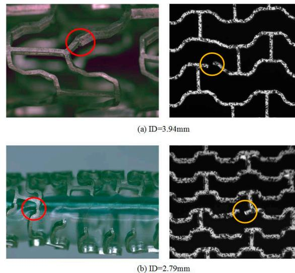
**Figure 17.** Fracture spots in the struts of stents with (a) Pattern B and (b) Pattern C in comparison with those in the planar specimens.
