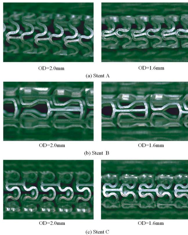
**Figure 12.** Experimental profiles of (a) Stent A, (b) Stent B, and (c) Stent C after crimping to outside diameters of 2.0 and 1.6 mm.
