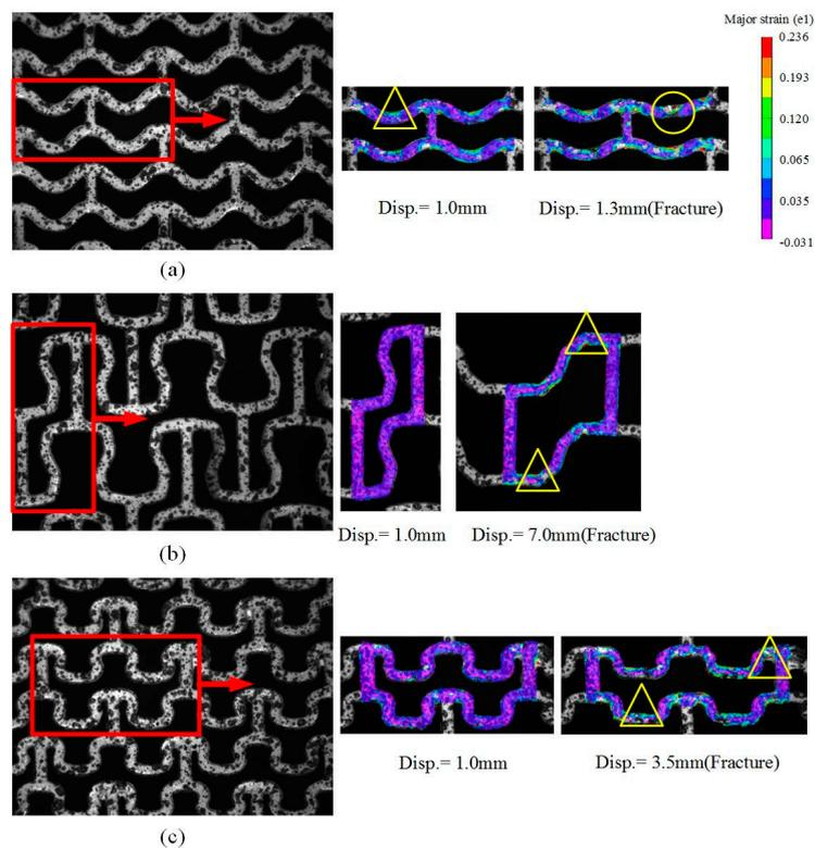
**Figure 9.** Speckle images and major strain distributions of the stent meshes during the stretching tests of the stents with: (a) Pattern A, (b) Pattern B, and (c) Pattern C. Triangle: strain concentration; Circle: Fracture.
