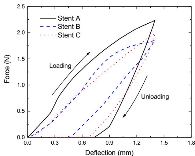
**Figure 21.** Three-point bending force-deflection curves of the three stents.
