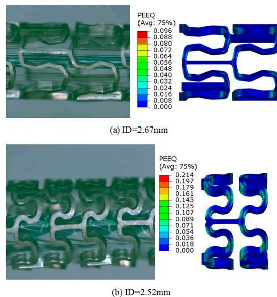
**Figure 16.** Experimental and simulated profiles of (a) Stent B and (b) Stent C expanded to the specific inside diameters.
