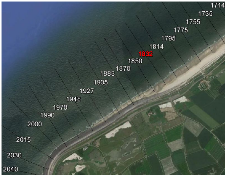
Figure 1.5: JARKUS transects at the Westkapelle sea defence, with transect 1832 shown in red. In this figure North is upward.
