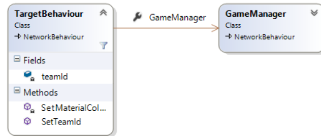
Figure 7.5: Overview of the target's code implementation in UML.
