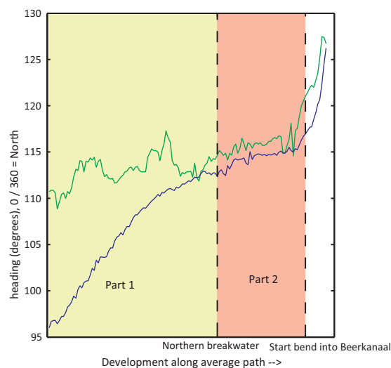
Figure 6.14 Development of the vessel heading under influence of a strong cross current (green) compared to the average heading (blue), both for vessels of size class 40,000-70,000 dwt
