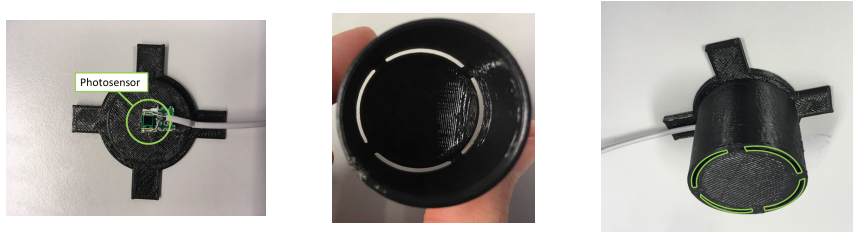
Figure 4.6: The left and middle figures show the bottom and cylinder parts of the aperture. The right most figure shows the resulting sensor, where the opening for the light rays is emphasized with the green lines.
