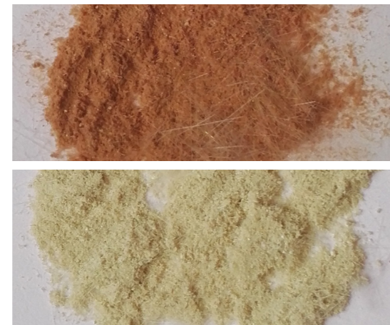
Figure 24 - Residue of PP (top) and PE (bottom) profiles
