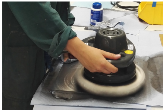
Figure 57 - Polishing the metal plates
