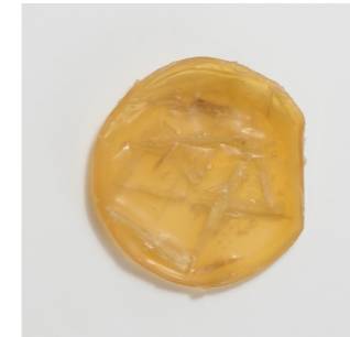
Latex with random oriented shredded composite
