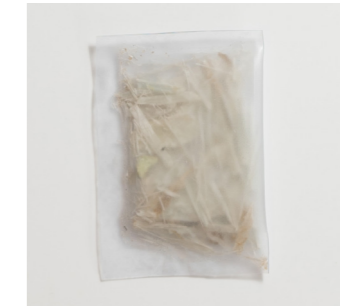
Shredded composite covered in plastic
