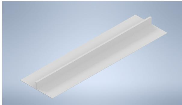
Figure 11.4: Plate-stiffener used in experiment
