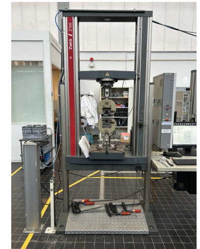
Figure 66 Compression Tests With The Universal Testing Machine Zwick Z100 (max. load 100kN)
