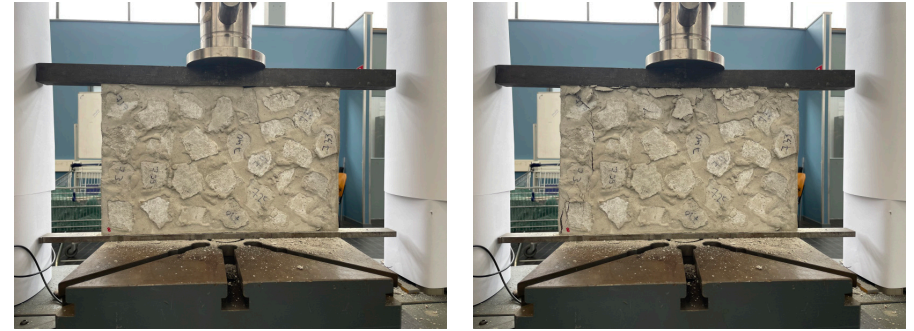
Figure 67 Wall 8 Before And After Compressive Failure
