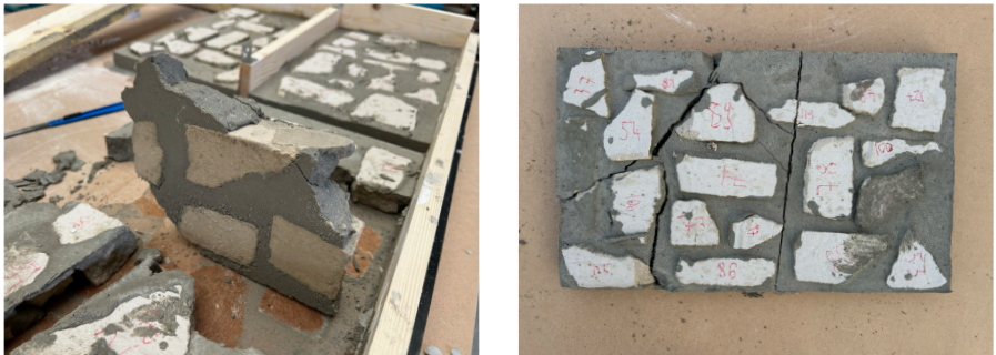
Figure 72 Breakage During Handling
