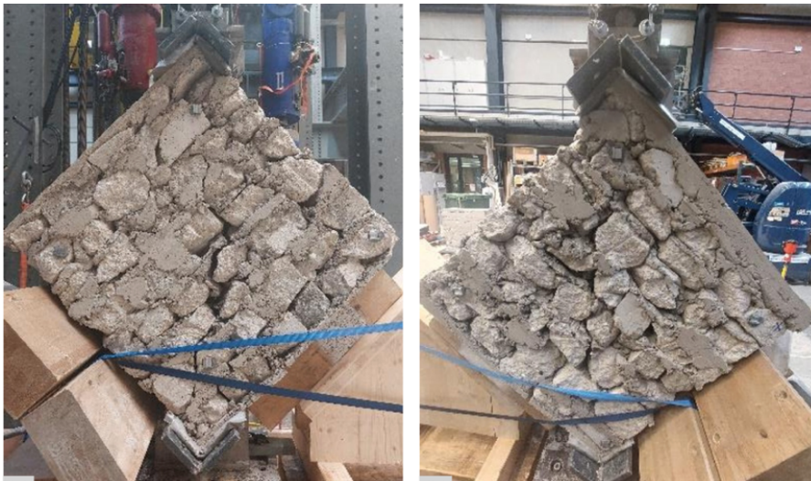
Figure 11 Wallets After The Diagonal Compression Tests (Oreb et al., 2024)
