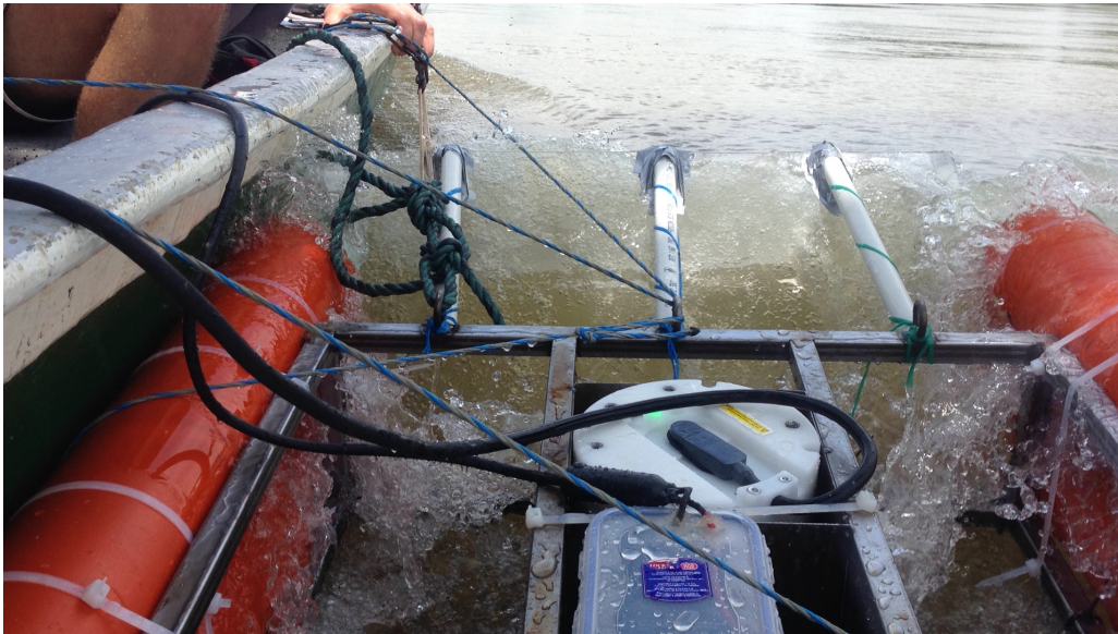
Figure C.3: Construction to stabilise the ADCP
