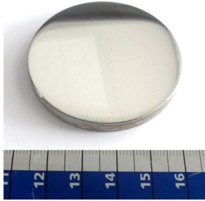
Figure 4.4: A mild steel surface after milling and polishing
