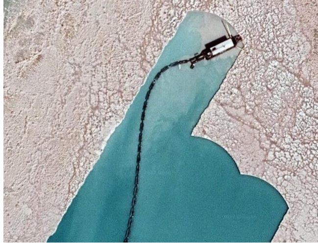
Figure 43: Closer aerial look of a Beaver 65 in operation
