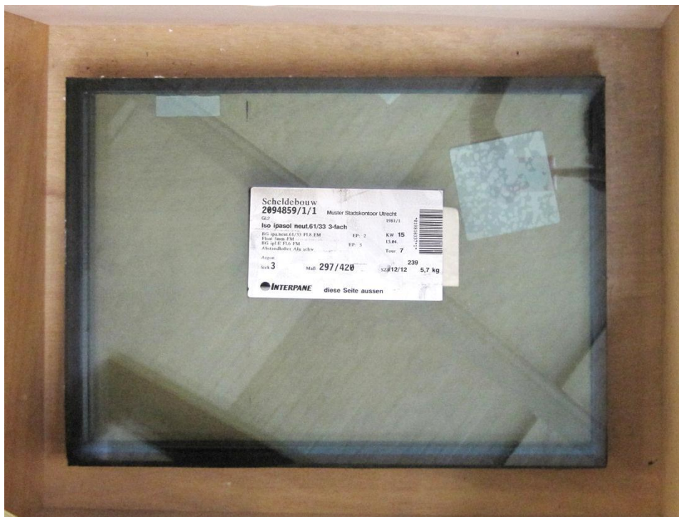
Figure 4.27 Testing element: a piece of triple glazing in A4 size
