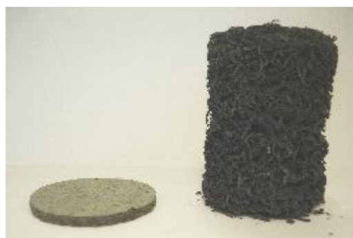
Figure 2.13 Intumescent tape before and after contact with fire
