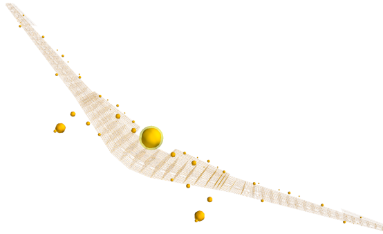
Figure 4.18: Mass model of the free-flying regional jet with no fuel inside the tanks
