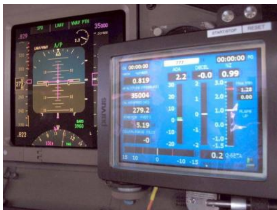
Figure 3.9: LADS installed next to the PFD[16].
