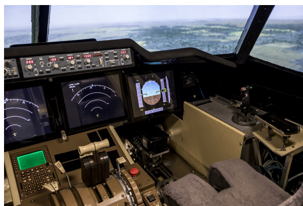
Figure 3.8: Experiment setup of Van Baelen, with side stick on the right[5].
