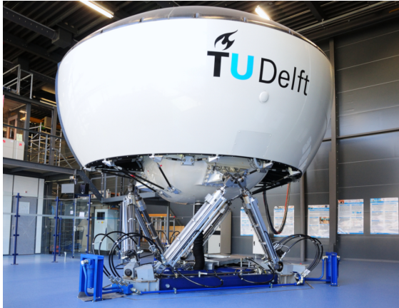
Fig. 10 Exterior of SIMONA at TU Delft.
