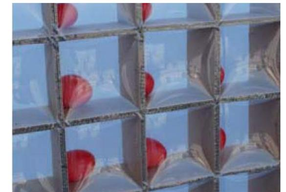
Figure 210: vacuum façade physical model (source: Knaack, U., Klein, T., Bilow, M., (2008), *Deflateables*, Rotterdam, 010 Publishers, p. 30)
