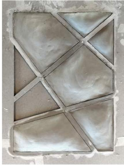
Figure 258: clay forming "bubbles" placed in the cardboard base
