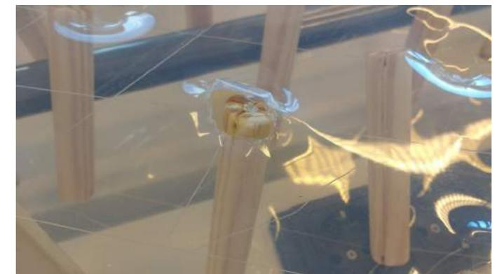
Figure 137: damage of the ETFE membrane
