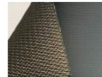
TENSOTHERM™ with nanogel® (layers with PTFE fiberglass)
