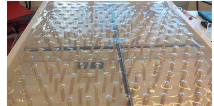
Figure 136: after the deflation and the damage of the membrane
