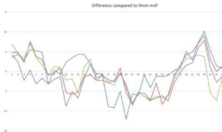
Figure 153: sound pressure levels differences compared to 9mm MDF plate
