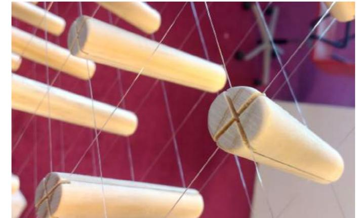
Figure 127: connection of the spacers with the wires
