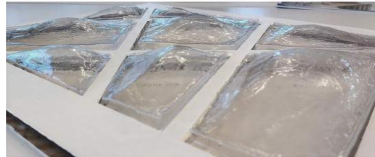
Figure 261: vacuum forming of a plastic sheet with clay as a mould
