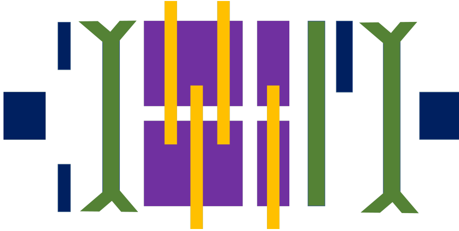
Figure 21: Schematic of the contacts of the device. The blue contacts are connected to the BLG. The purple contacts represent the large (left) and small (right) set of split gates. The green contacts are the other top gates on top of the hBN. The finger gates are represented by the yellow rectangles.
