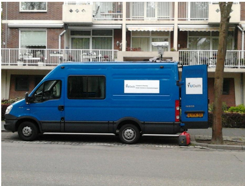
Figure 4-1 Video observation van with camera on top
