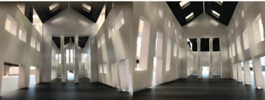
daylighting with transparent opening on the side of the new roof
