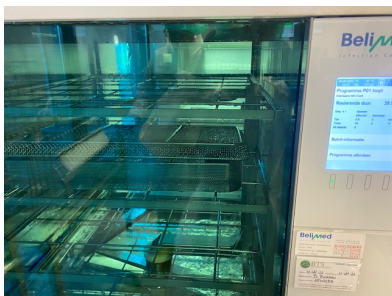
(c) The four test objects in the washer-disinfector
