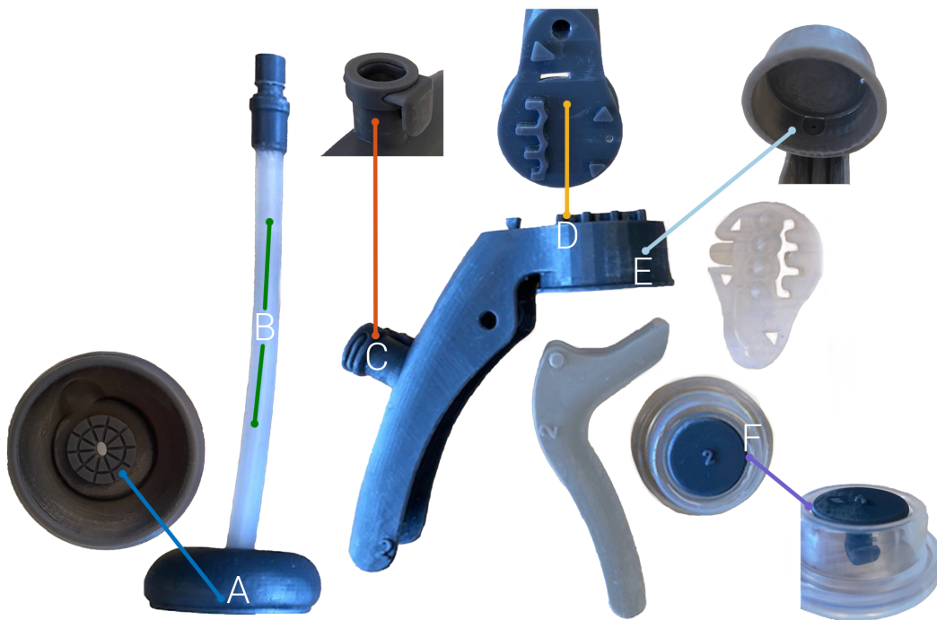
Fig. 4.3.: Indication of the six different test locations. A: Inside the cup. B: Inside the tube. C: Connection from the handle to the tube. D: Above the head of the handle. E: Under the head of the handle. F: Between the stem and diaphragm. The back handle and the silicone domes are transparent, as no specific test locations have been chosen for these parts.
