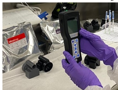
(f) Reading results from the ATP monitor.
