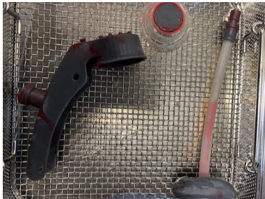
(a) The vela's are soiled after one cycle in the washer-disinfector.
