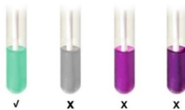
Fig. 2.2.: The four potential color outcomes resulting from the protein test. Any color except green indicates contamination, image from [32].
