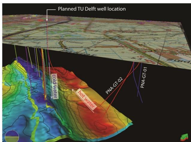
**Figure 2: 3D structural model of the DSSM in the study area with trajectories of the planned TU Delft geothermal wells. Wells PNA-GT-01 and PNA-GT-02: producing geothermal doubles.**
