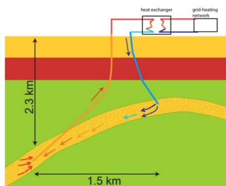
**Figure 3: Schematized view of the design of a doublet for production of geothermal energy from an aquifer. A deviated well is used to produce water with a temperature of 65-75 °C from the aquifer at two kilometers depth. At the surface heat is extracted by a heat exchanger to a local grid to sustainably heat buildings and greenhouses. A second well re-injects the cooled-down aquifer water into the same reservoir rock two kilometers away from the production point.**
