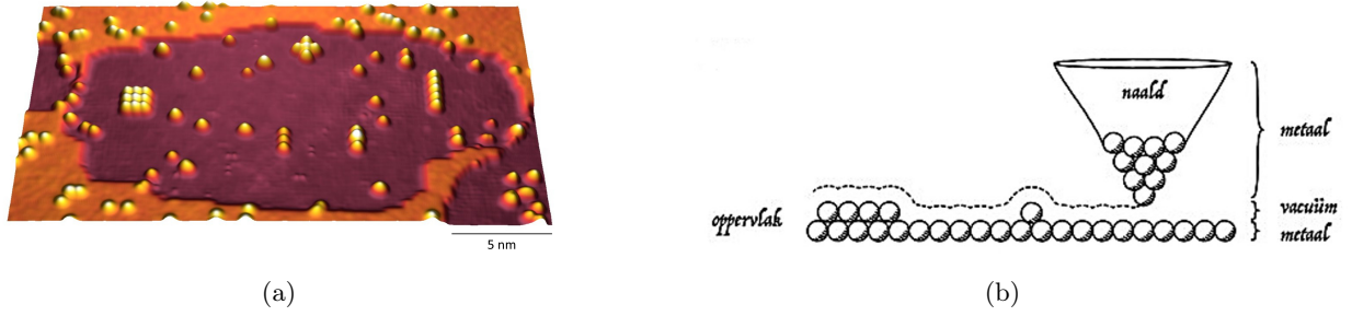
Figure 1.2: (a) STM image showing the construction of atomic structures of Fe on \text{Cu}_2\text{N}/\text{Cu}(100) on a 30 nm scale. (b) Illustration of STM scanning a surface at atomic resolution. Source: OtteLab [2].
