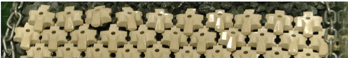
Figure A.5 : Start of damage and failure, end test 2.1
