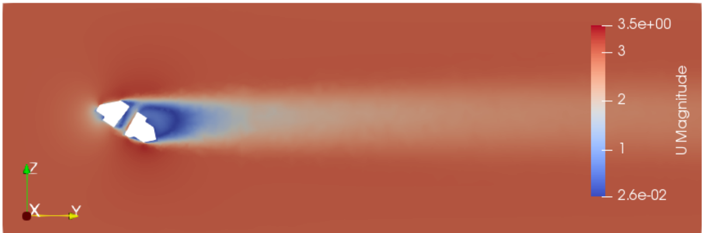
Figure 35: Velocity in the YZ domain, incoming velocity in positive Y direction (3 m/s), cross section through half of the block width
