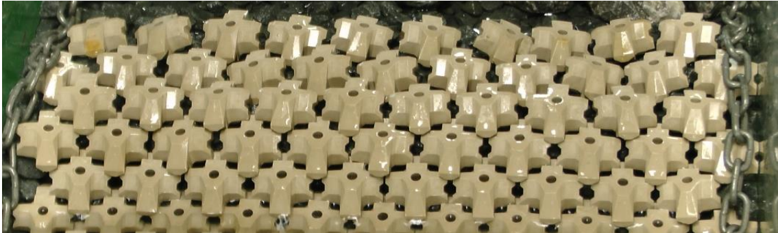
Figure A.12: Start of damage, end test 5.2
