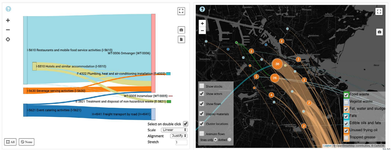
Figure 3.2. AS-MFA module in the GDSE. The Sankey diagram on the left represents material flows between different economic activities, and the map on the right represents the same flows on a map. The flows can be toggled on and off by using the interactive Sankey diagram (source: GDSE, REPAiR 2018)
