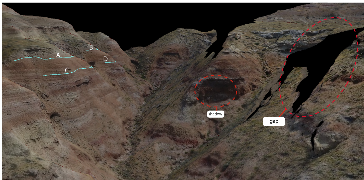
Figure 3.3: An example of two flaws in the photopanel. On the left is shadow, making the outcrop less clearly visible. On the right is a gap in the data. The example is from one of the sidecanyons in panel 13. Note that the gap can be prevented by better drone photography, while the shadow is weather dependent. Lines A to D partly mark two succession boundaries, to indicate the methodology. All other succession boundaries are not shown in the figure.
