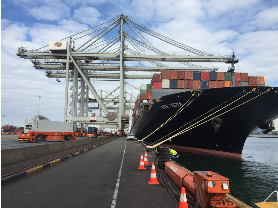
Figure 4: Shore tension applied at Delta Terminal (Photo PoR-Erik Broos)
