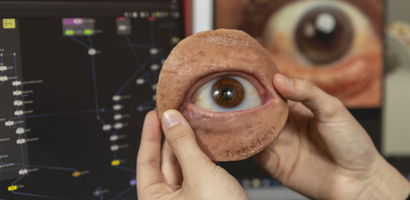
Figure 27. Voxel printing for ocular prosthetics
